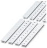
Zack marker strip, Can be ordered: Strip, white, Labeled according to customer specifications, Mounting type: Snap into tall marker groove, For terminal block width: 10.2 mm, Lettering field: 10.15 x 10.5 mm
