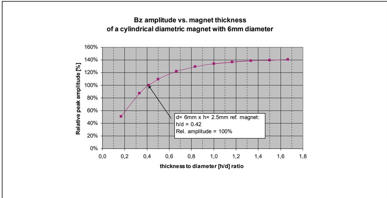
As the graph in Figure 15 shows, the amplitude drops significantly at h/d ratios below this value and remains relatively flat at ratios above 1.3.
