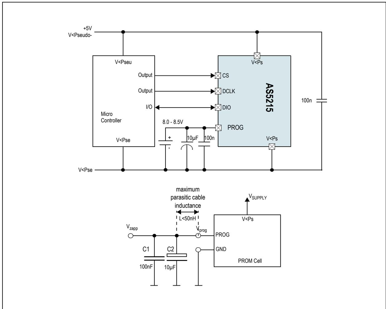
For programming of the OTP, an additional voltage has to be applied to the pin PROG. It has to be buffered by a fast 100nF capacitor (ceramic) and a 10µF capacitor. The information to be programmed is set by command 25. The OTP bits 16 until 45 are used for ams OSRAM factory trimming and cannot be overwritten.
