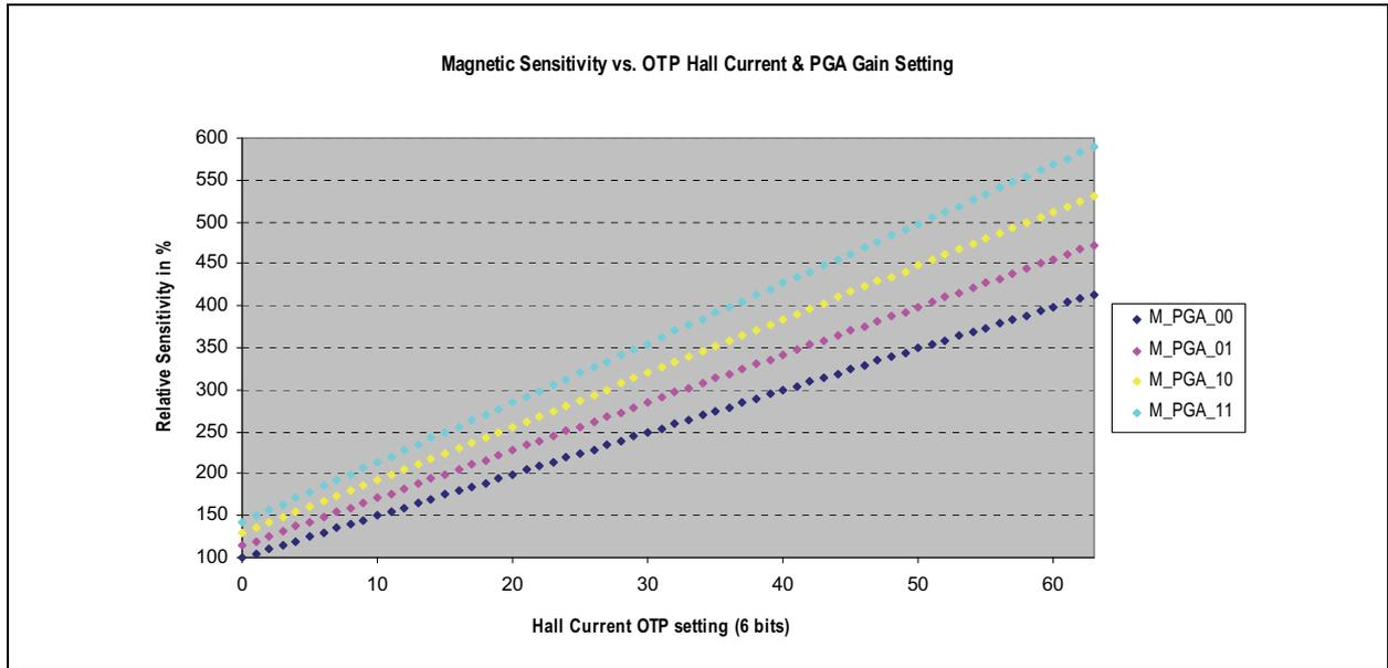
The amplitude of the output signal is programmable via sensitivity (6bit) and/or gain (2bit) settings (see Figure 25).
