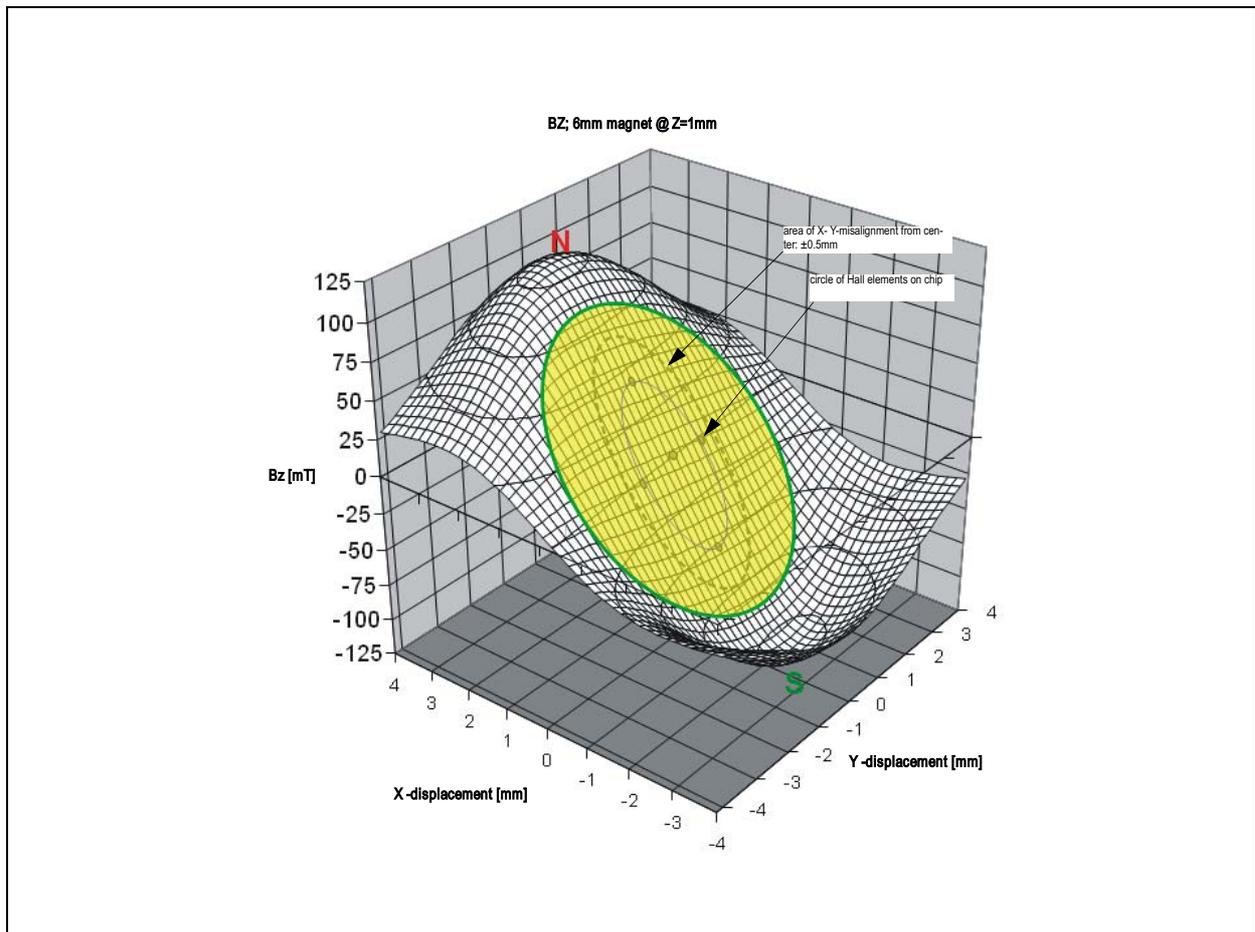
As shown in Figure 14 (grey zone), the Hall elements are located on the chip at a circle with a radius of 1mm. Since the difference between two opposite Hall sensors is measured, there will be no difference in signal amplitude when the magnet is perfectly centered or if the magnet is misaligned in any direction as long as all Hall elements stay within the linear range.
