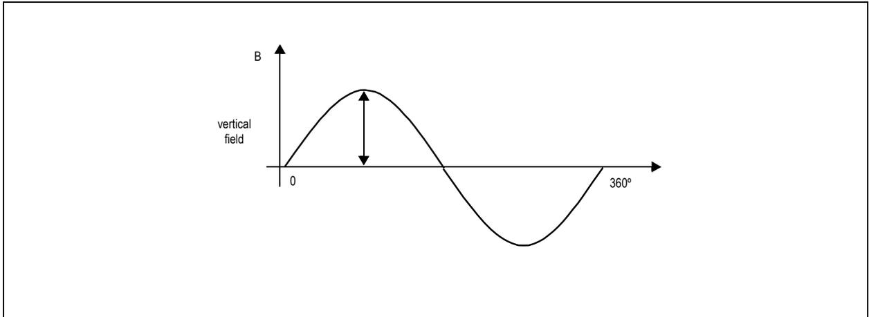
The recommended magnetic field, measured at the chip surface on a radius equal to the Hall sensor array radius (typ 1mm) should be within a certain range. This range lies between 45 and 75mT or between 20 and 80mT, depending on the encoder product.
