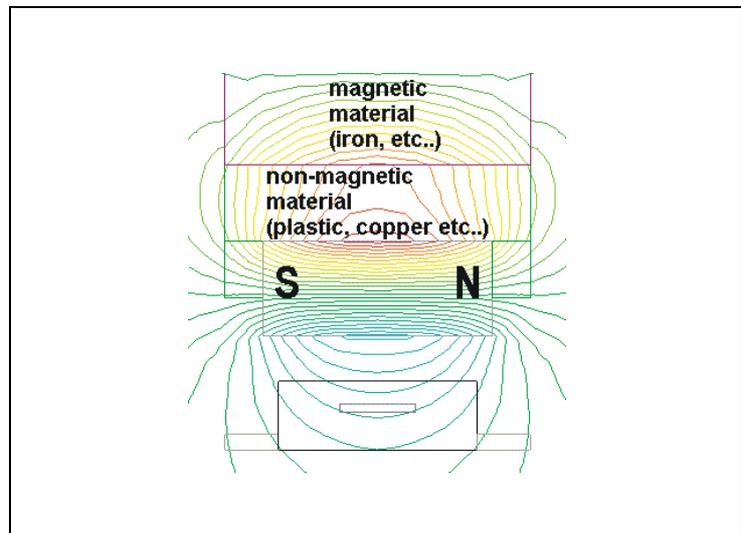
If the magnet has to be mounted inside a magnetic shaft, a possible solution is to place a non-magnetic spacer between shaft and magnet, as shown in [Figure 20](#). While the magnetic field is rather distorted towards the shaft, there are still adequate field lines available towards the sensor IC. The distortion remains reasonably low.
