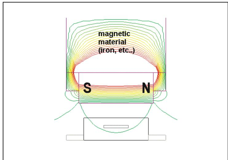
If the magnet is mounted in a ferromagnetic material, such as iron, most of the field lines are attracted by the iron and flow inside the metal shaft (see Figure 19). The magnet is weakened substantially.
