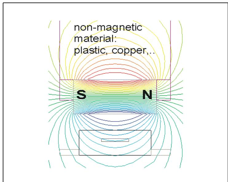
If the magnet is mounted in non-magnetic material, such as plastic or diamagnetic material, such as copper, the magnetic field distribution is not disturbed. Even paramagnetic material, such as aluminium may be used. The magnet may be mounted directly in the shaft (see Figure 18).
