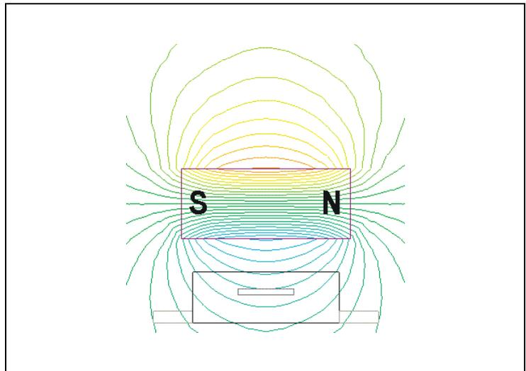
Figure 17 shows the ideal case with the magnet in air. No magnetic materials are anywhere nearby.
