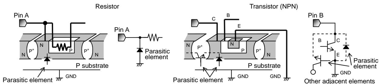
Fig.42 Simplified structure of monoristic IC
