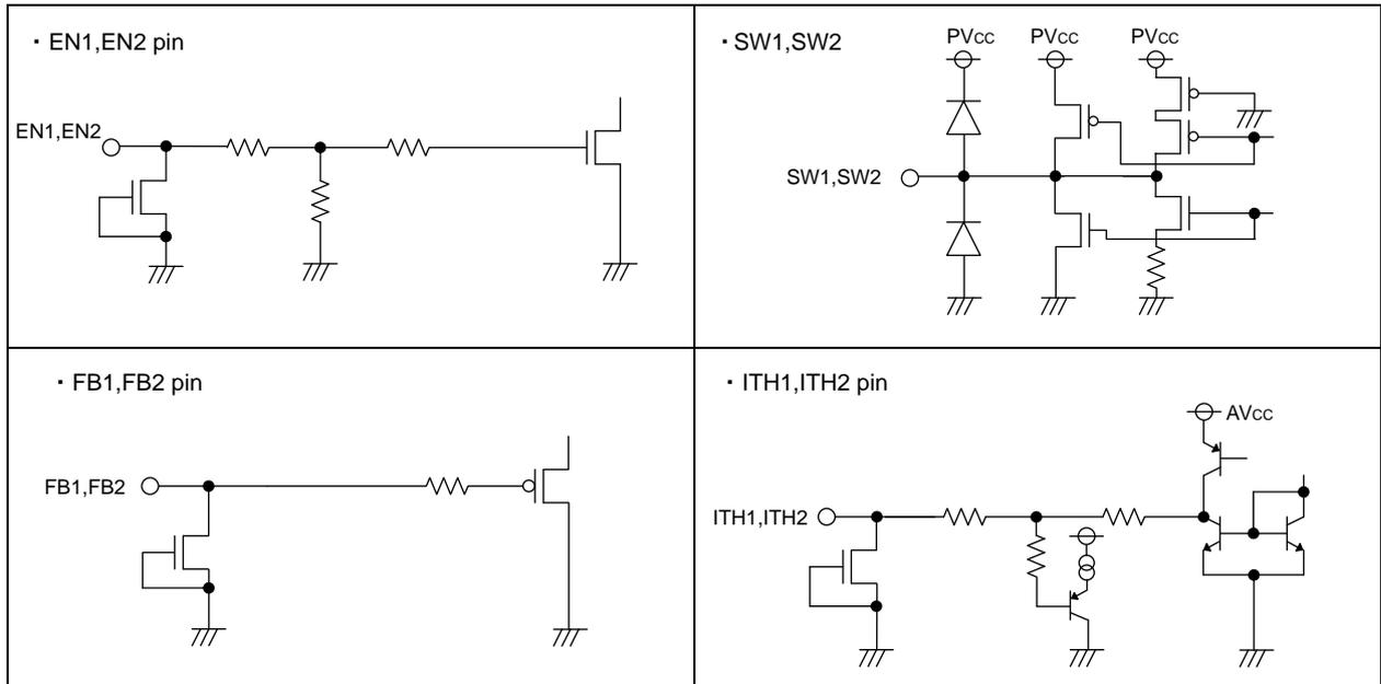
Fig.41 I/O equivalence circuit
