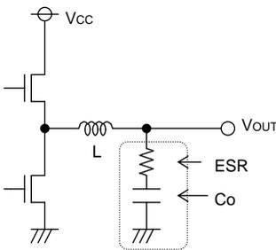
Fig.34 Output capacitor
