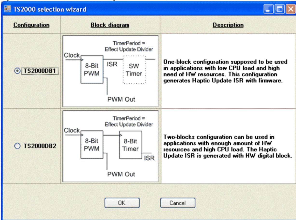
Figure 8. TS2000 User Module Configurations Selection, CY8C20xx6H Devices
