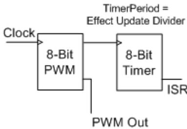
Figure 3. TS2000 Haptics Block Diagram. One Digital Block Configuration, Direct Update Method Option
