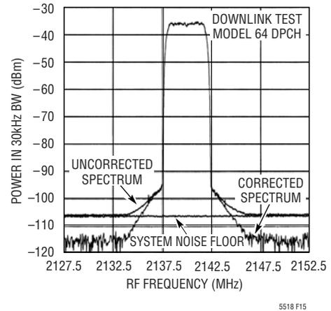
**Figure 15. 1-Channel W-CDMA Spectrum**
