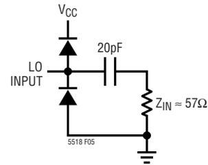
Figure 5. Equivalent Circuit Schematic of the LO Input
