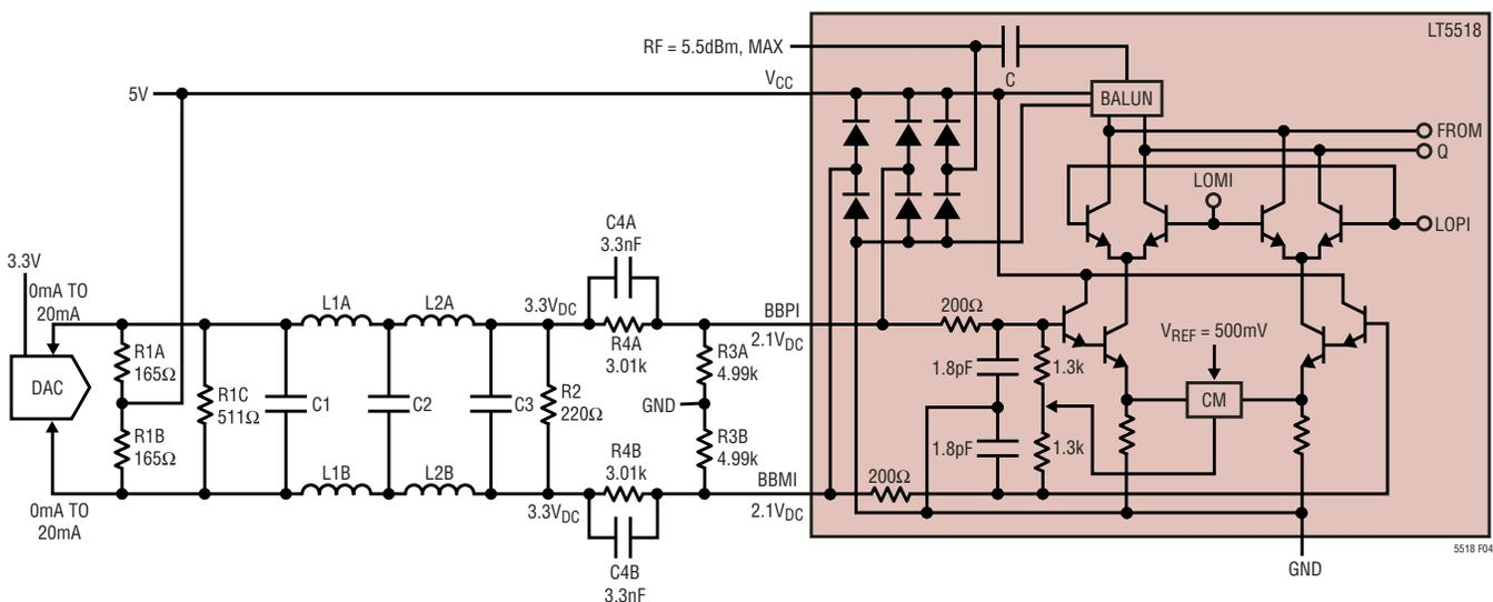
Figure 4. LT5518 5th Order Filtered Baseband Interface with 3.3V<sub>CM</sub> DAC (Only I-Channel is Shown).
