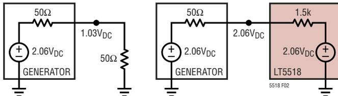
**Figure 2. DC Voltage Levels for a Generator Programmed at 1.03V<sub>DC</sub> for a 50Ω Load and for the LT5518 as a Load**
