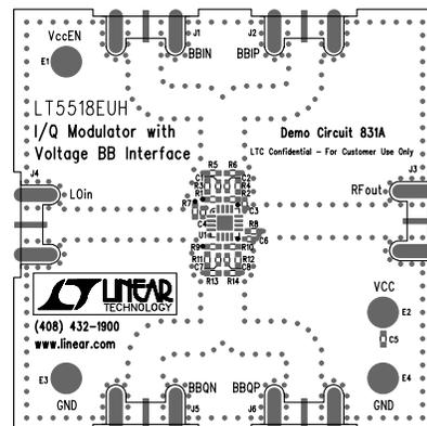
Figure 10. Component Side Silk Screen of Demo Board
