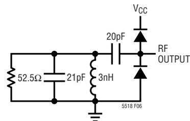
**Figure 6. Equivalent Circuit Schematic of the RF Output**
