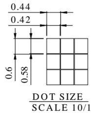
The non-specified tolerance of dimension is ±0.3mm.
