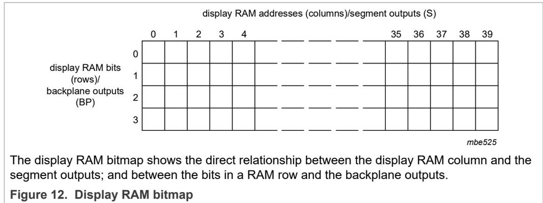
When display data is transmitted to the PCA85176, the display bytes received are stored in the display RAM in accordance with the selected LCD drive mode. The data is stored as it arrives and depending on the current multiplex drive mode the bits are stored singularly, in pairs, triples, or quadruples. To illustrate the filling order, an example of a 7-segment display showing all drive modes is given in [Figure 13](#); the RAM filling organization depicted applies equally to other LCD types.
