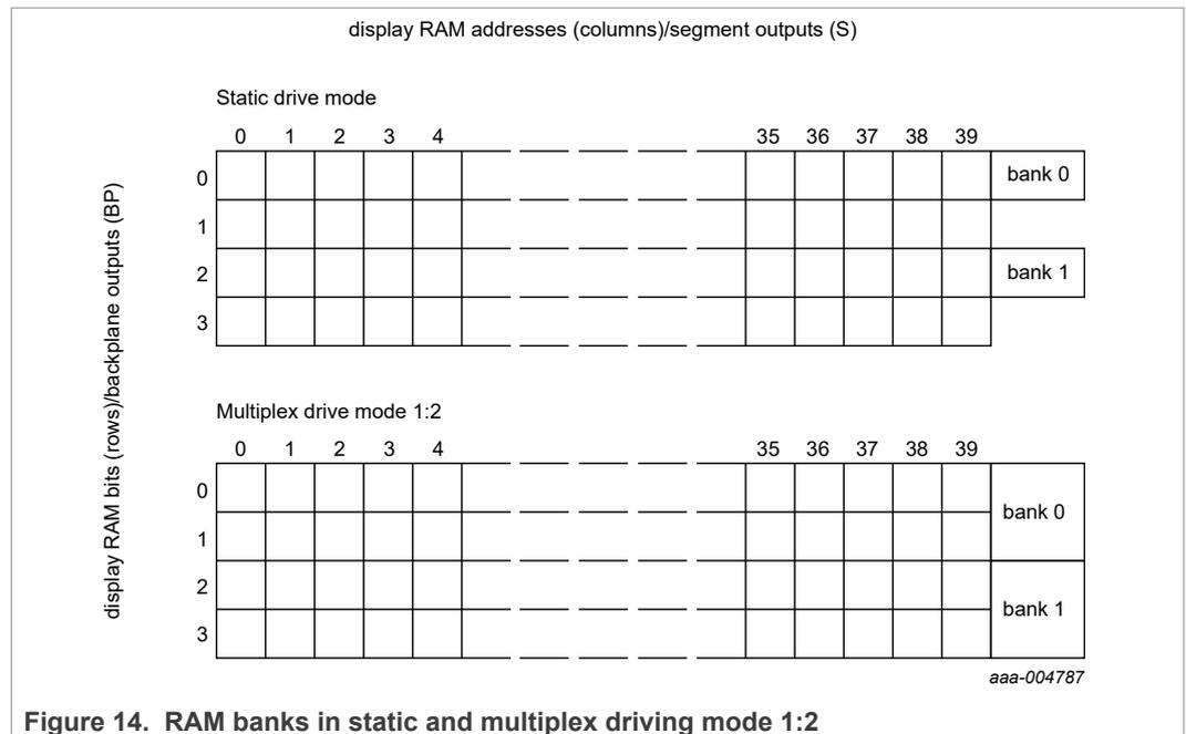
Figure 14. RAM banks in static and multiplex driving mode 1:2
