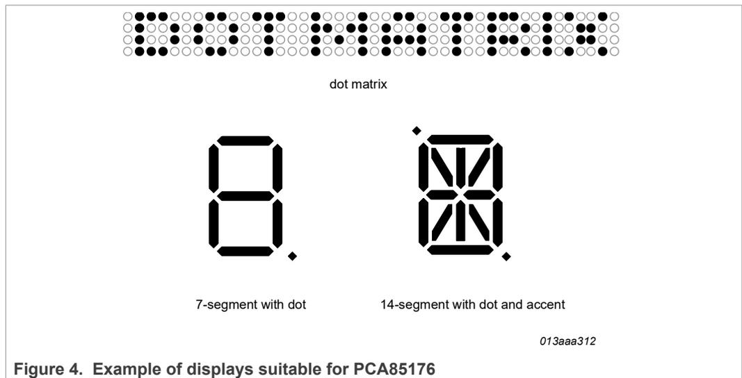
Figure 4. Example of displays suitable for PCA85176
