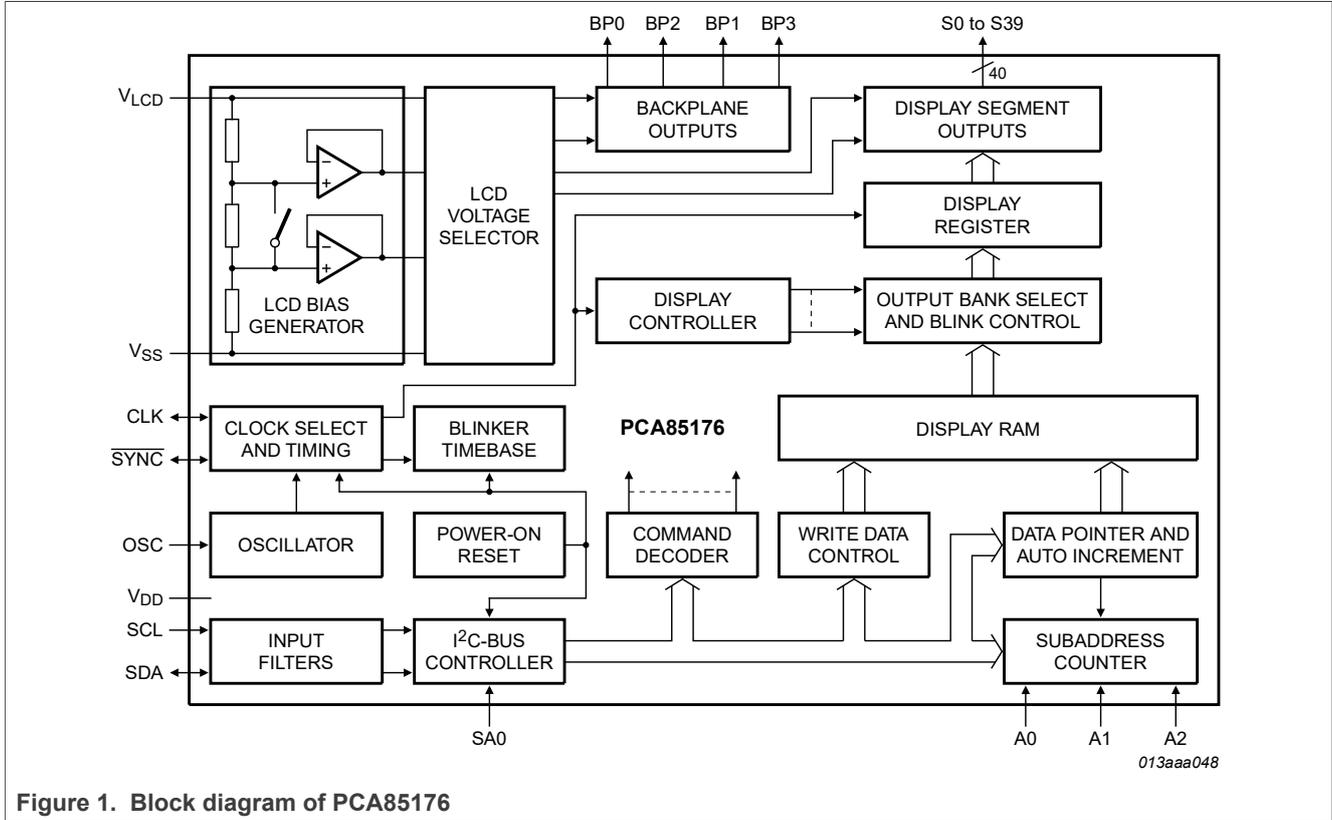
Figure 1. Block diagram of PCA85176
