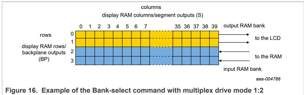
Figure 16. Example of the Bank-select command with multiplex drive mode 1:2
