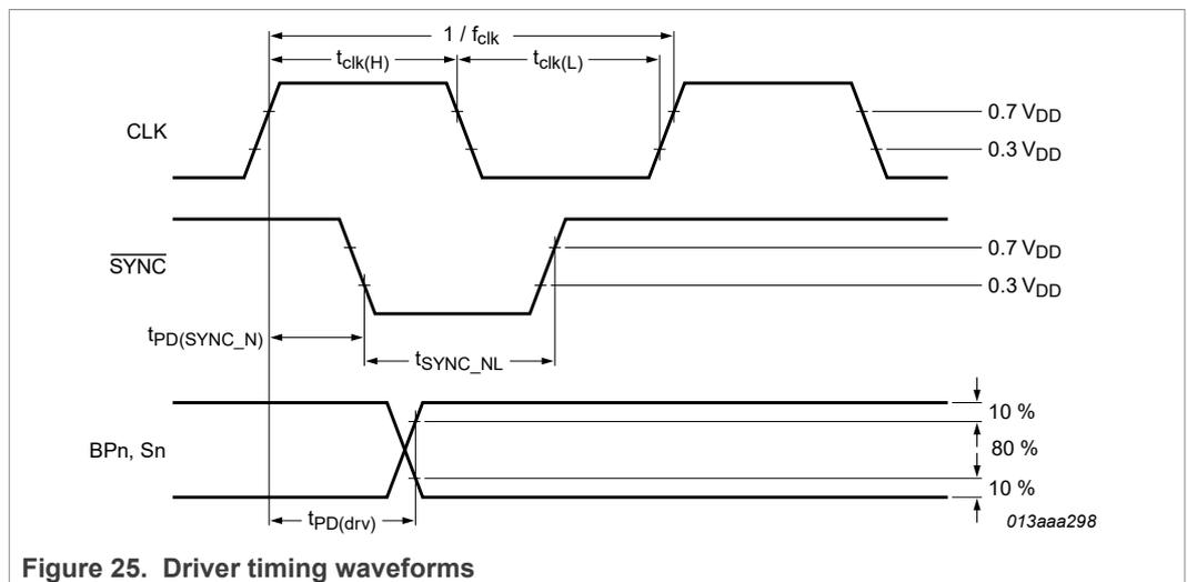
Figure 25. Driver timing waveforms
