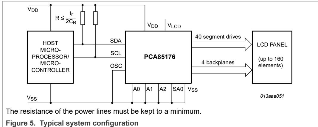
The host microcontroller maintains the 2-line I<sup>2</sup>C-bus communication channel with the PCA85176. The internal oscillator is enabled by connecting pin OSC to pin V<sub>SS</sub>. The appropriate biasing voltages for the multiplexed LCD waveforms are generated internally. The only other connections required to complete the system are the power supplies (V<sub>DD</sub>, V<sub>SS</sub>, and V<sub>LCD</sub>) and the LCD panel chosen for the application.
