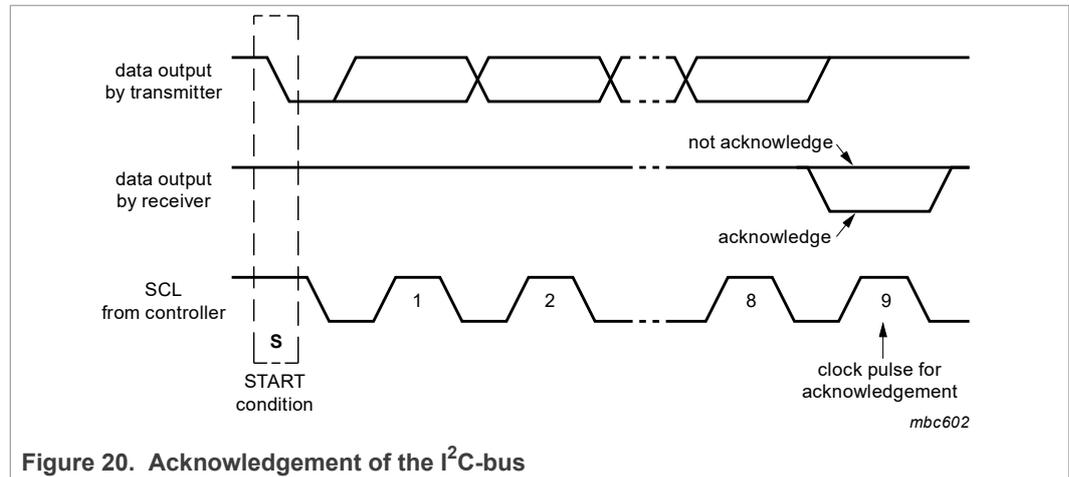
Figure 20. Acknowledgement of the I<sup>2</sup>C-bus
