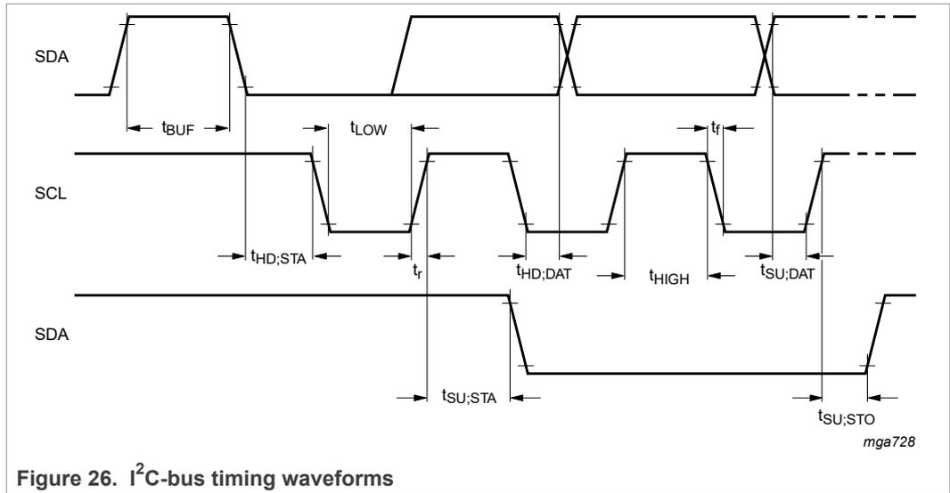
Figure 26. I<sup>2</sup>C-bus timing waveforms
