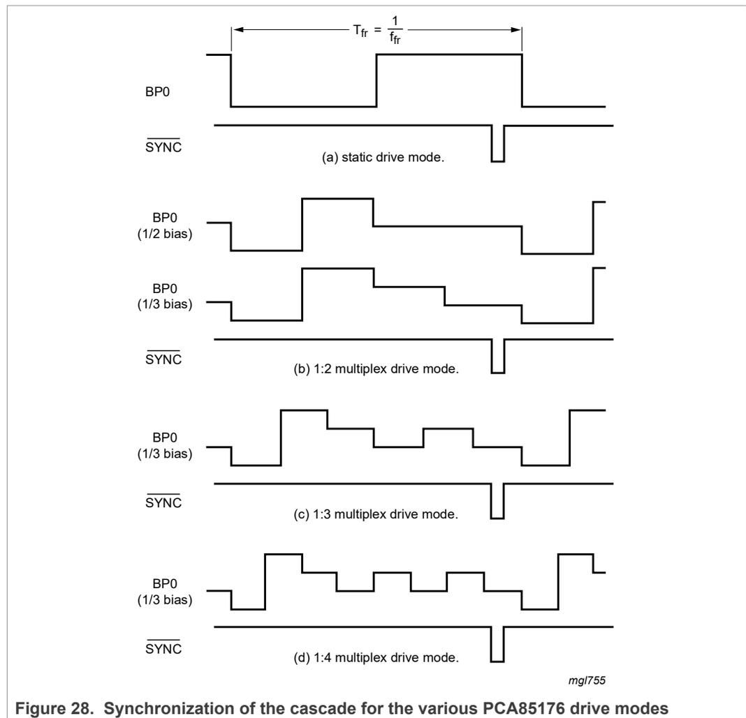
Figure 28. Synchronization of the cascade for the various PCA85176 drive modes
