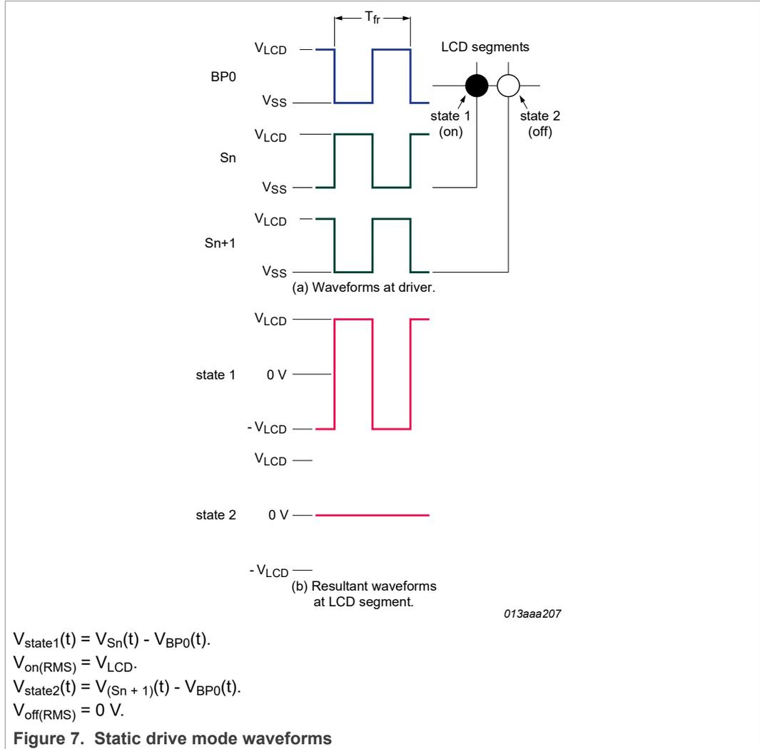
Figure 7. Static drive mode waveforms
