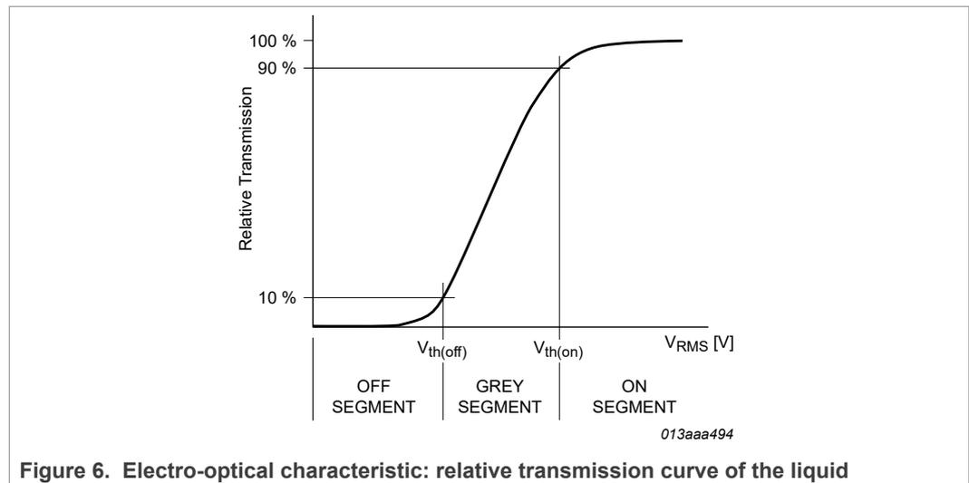
Figure 6. Electro-optical characteristic: relative transmission curve of the liquid
