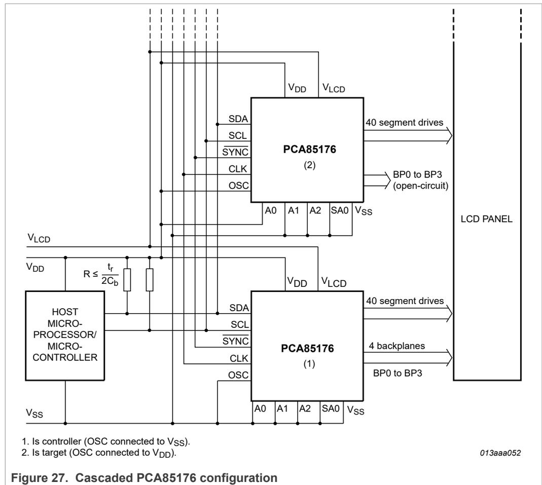
Figure 27. Cascaded PCA85176 configuration
