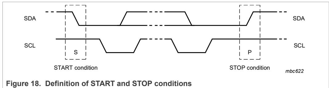
Figure 18. Definition of START and STOP conditions
