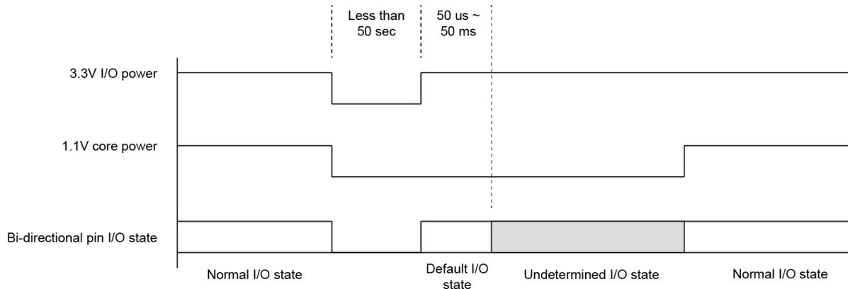
**Figure 14-1 Timing Sequence with Undetermined I/O State**
