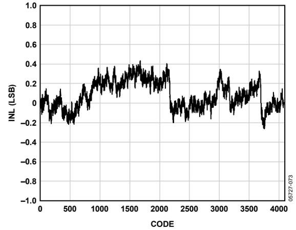
Figure 37. INL,  $f_{IN} = 2.4$  MHz,  $f_{SAMPLE} = 65$  MSPS
