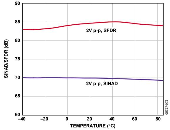
Figure 36. SINAD/SFDR vs. Temperature,  $f_{IN} = 10.3$  MHz,  $f_{SAMPLE} = 65$  MSPS
