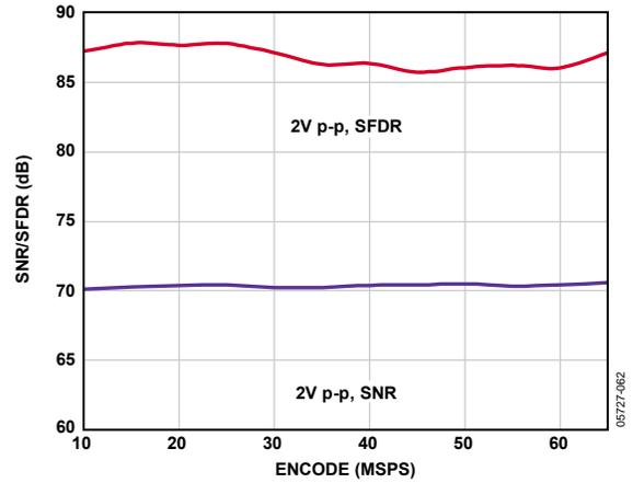
Figure 25. SNR/SFDR vs. Encode,  $f_{IN} = 10.3$  MHz,  $f_{SAMPLE} = 65$  MSPS
