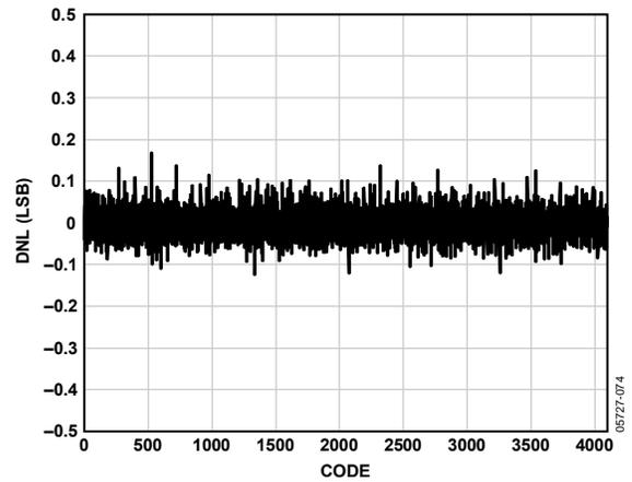
Figure 38. DNL,  $f_{IN} = 2.4$  MHz,  $f_{SAMPLE} = 65$  MSPS
