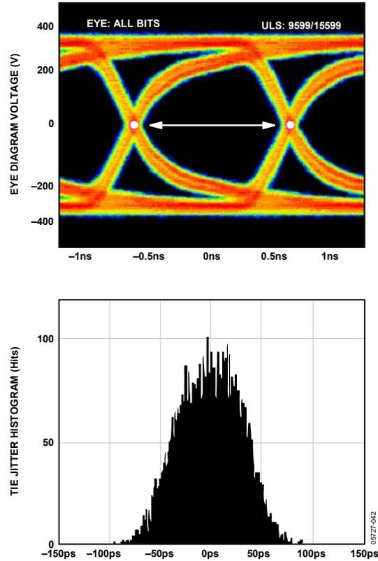
Figure 63. Data Eye for LVDS Outputs in ANSI-644 Mode with 100  $\Omega$  Internal Termination on and Trace Lengths Greater than 24 Inches on Standard FR-4, External 100  $\Omega$  Far Termination Only
