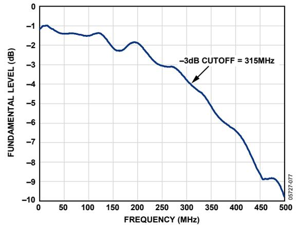
Figure 42. Full-Power Bandwidth vs. Frequency,  $f_{SAMPLE} = 65$  MSPS
