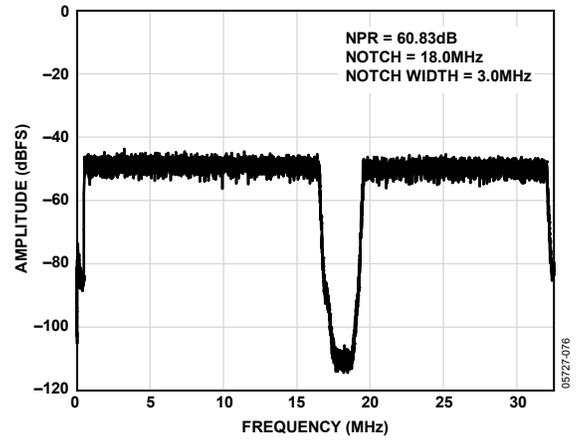
Figure 41. Noise Power Ratio (NPR),  $f_{SAMPLE} = 65$  MSPS
