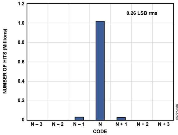
Figure 40. Input-Referred Noise Histogram,  $f_{SAMPLE} = 65$  MSPS
