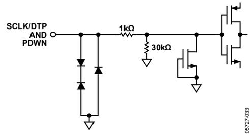
Figure 10. Equivalent SCLK/DTP and PDWN Input Circuit
