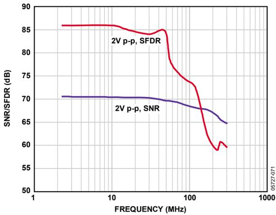
Figure 35. SNR/SFDR vs. Frequency,  $f_{SAMPLE} = 65$  MSPS
