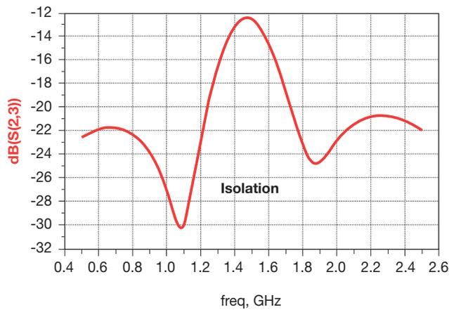
**Note:** Measurements were taken using an Anritsu 4 port VNA; Diplexer was mounted on a custom evaluation board. To reduce systematic errors from the VNA, the coaxial measurement cables, and evaluation board, a Short-Open-Load-Thru (SOLT) calibration was performed, using a custom fabricated calibration substrate. This is the most common coaxial calibration methods.
