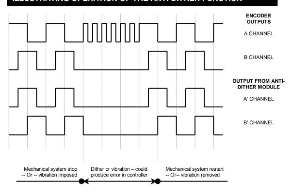
Note: For simplicity of illustration, the inverted channels, A/ and B/ have not been shown. The index, or Z, channel is also not shown in the above diagram but is passed through directly as an optically isolated signal and maintains its original relationship to the encoder output channel. Reference http://www.beisensors.com/pdfs/oim.pdf for connection diagrams.
