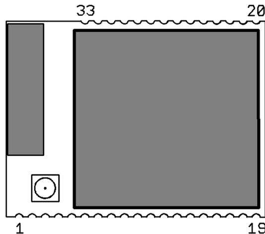
**Figure 1: ETRX3 series Module Pinout (top view)**
