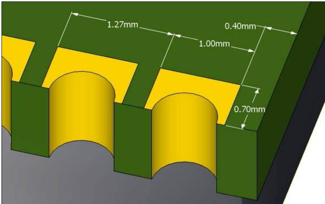
Figure 6. Typical pad dimensions
