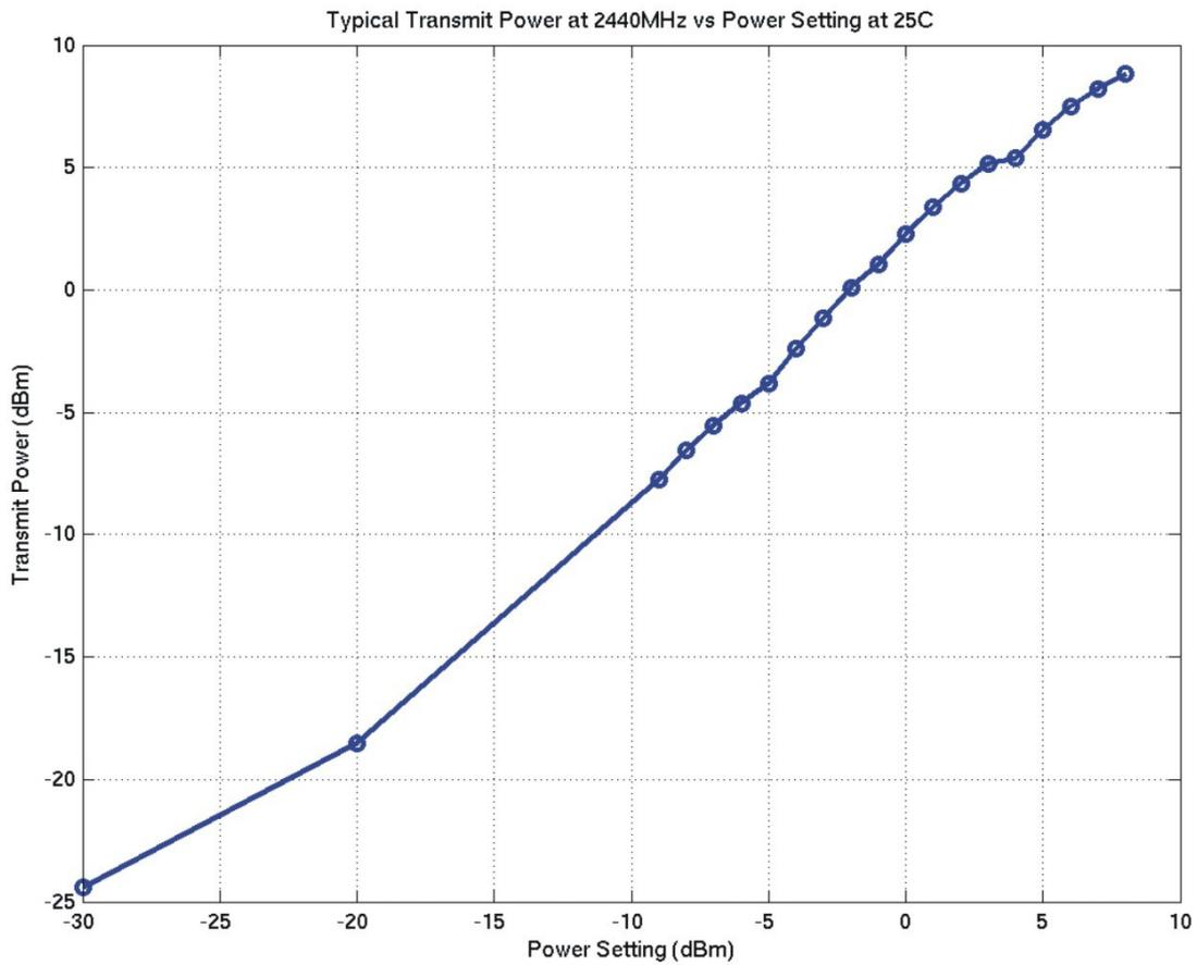
Figure 3: Output Power vs. Power Setting
