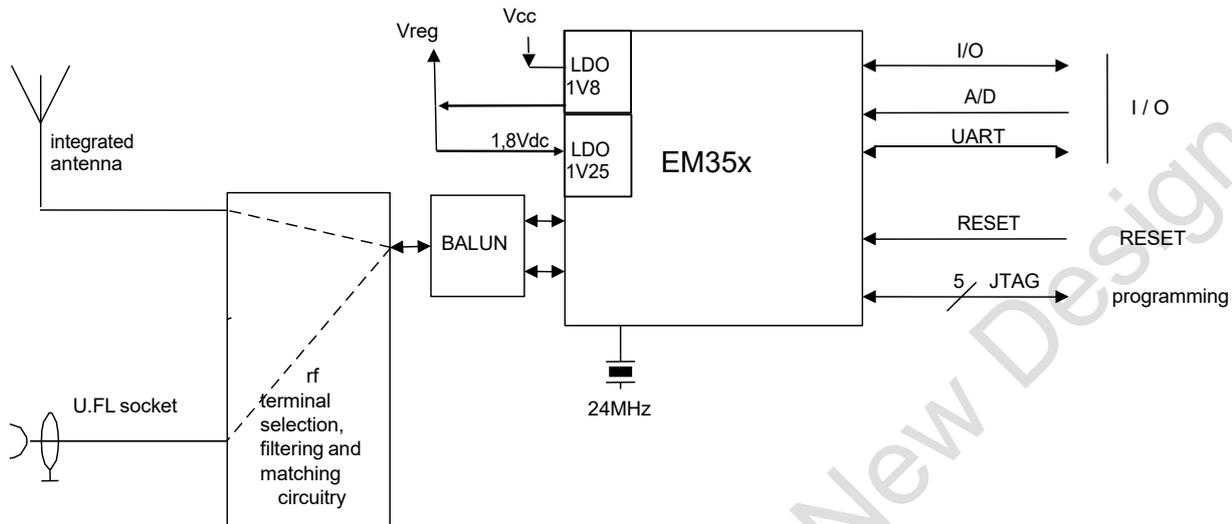
Figure 2: Hardware Diagram
