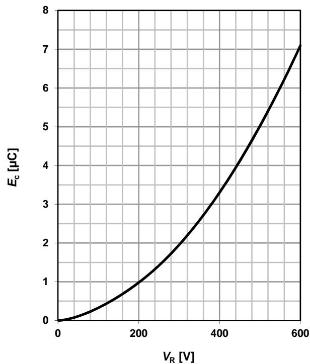
**10 Typ. capacitance charge vs. current slope**
