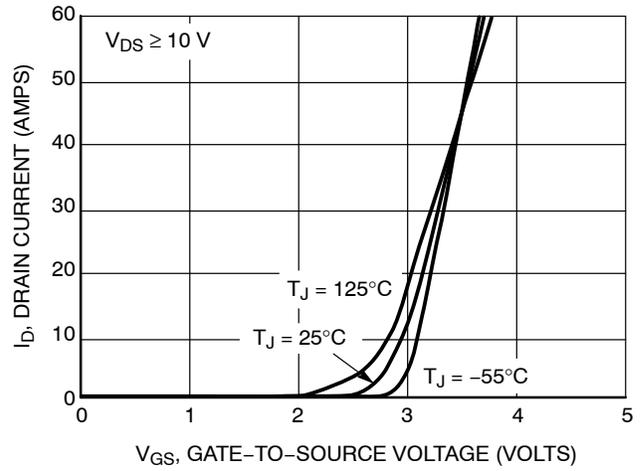
**Figure 2. Transfer Characteristics**
