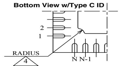
There are 3 methods of indicating pin 1 corner at the back of the VFQFN package are:
