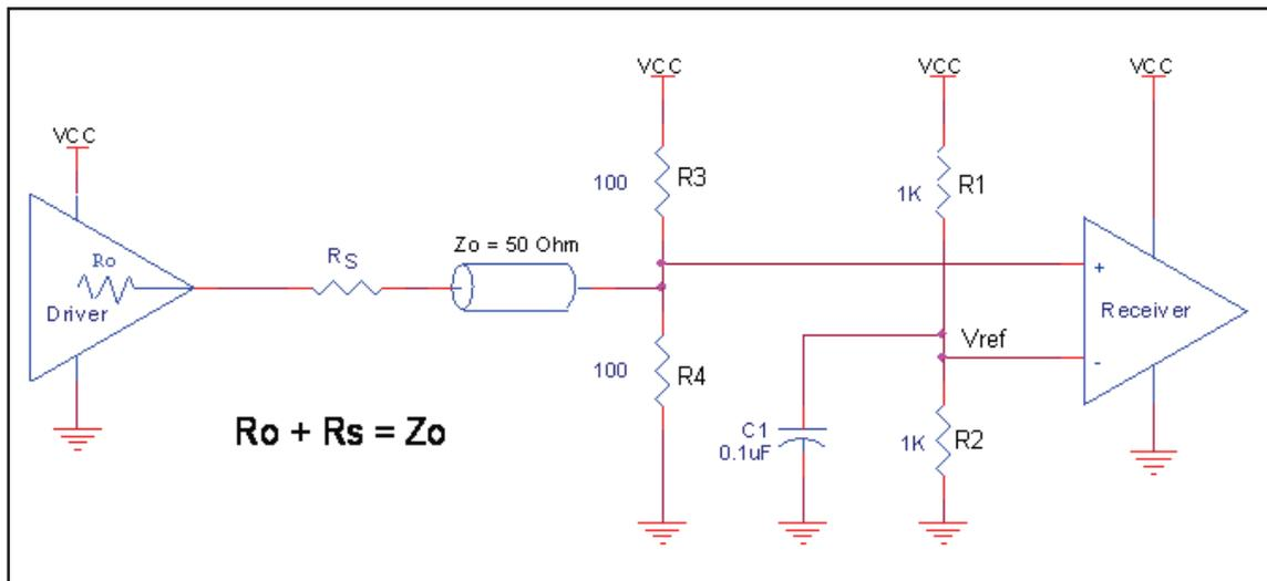
FIGURE 2. SINGLE ENDED SIGNAL DRIVING DIFFERENTIAL INPUT
