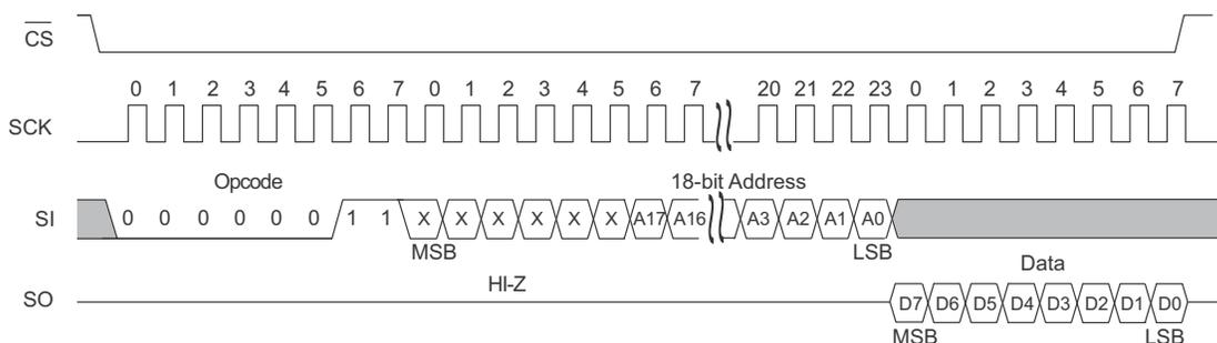
**Figure 12. Fast Read Operation**
