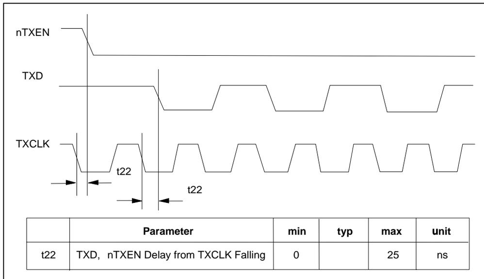
Figure 12.18 – External ENDEC Interface – Start of Transmit
