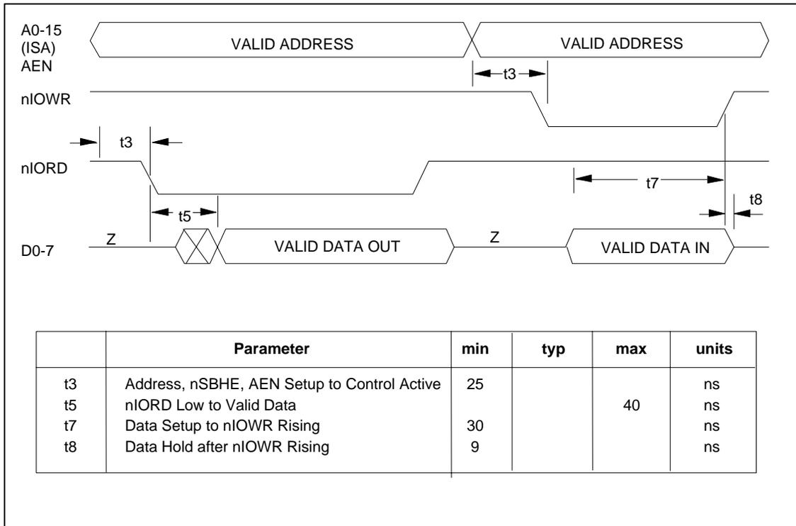
Figure 12.9 - 8-Bit Mode Register Cycles
