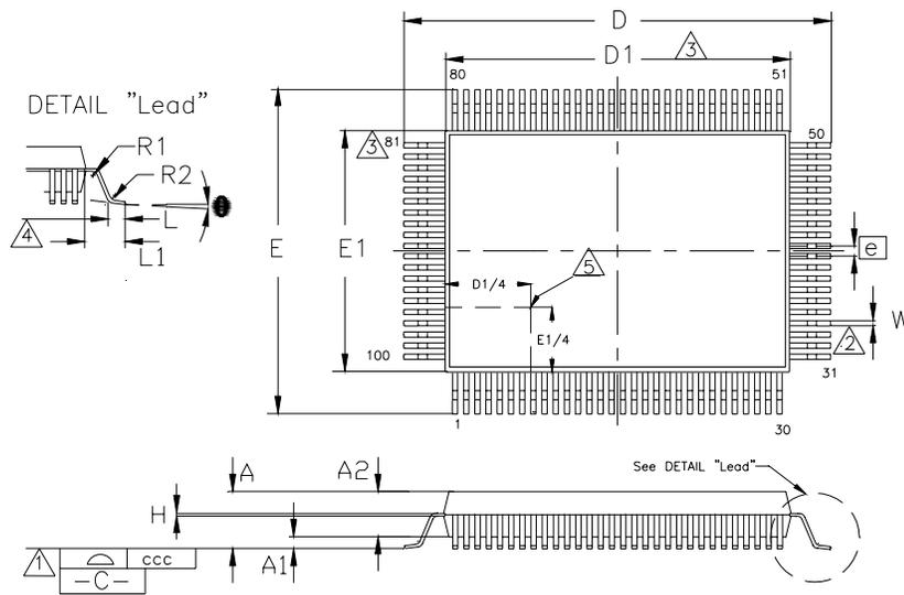
Figure 12.28 - 100 PIN QFP Package
