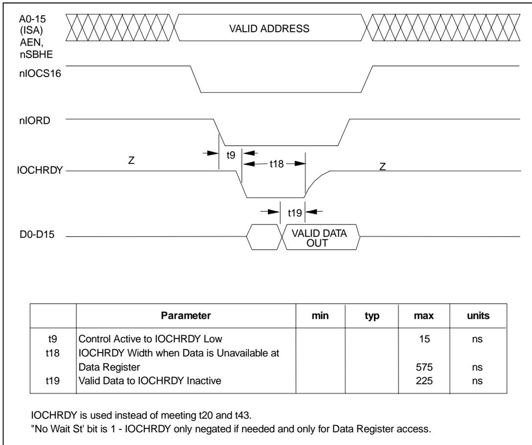
Figure 12.7 – Data Register Special Read Access
