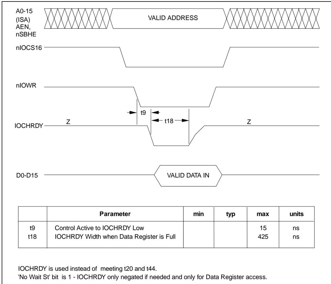
**Figure 12.8 – Data Register Special Write Access**
