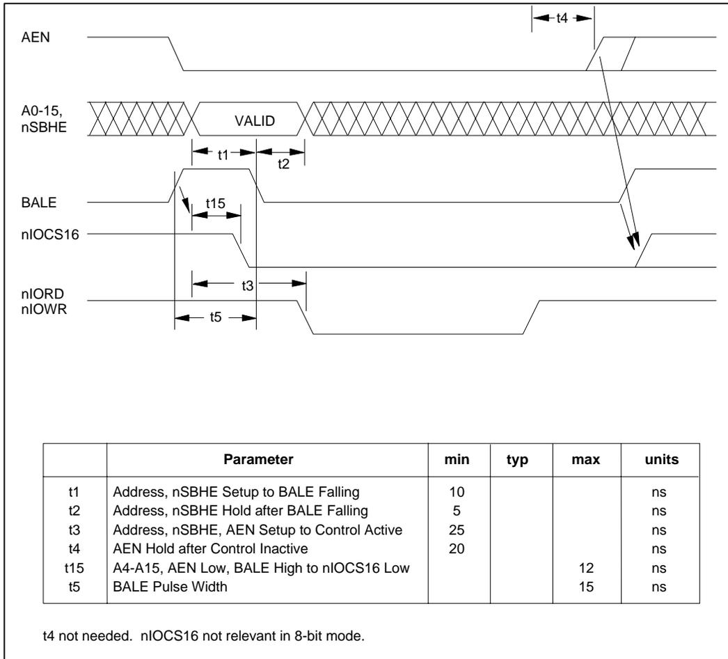
Figure 12.13 – Local Bus Register Access When Using Bale
