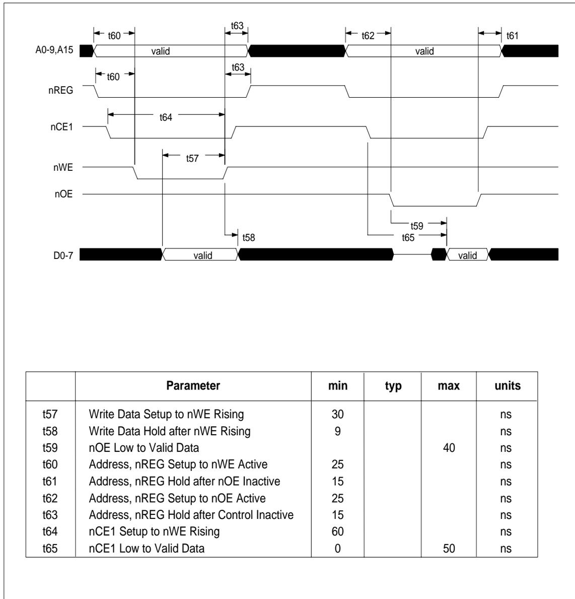
Figure 12.1 – Card Configuration Registers – Read/Write PCMCIA Mode (A15=1)
