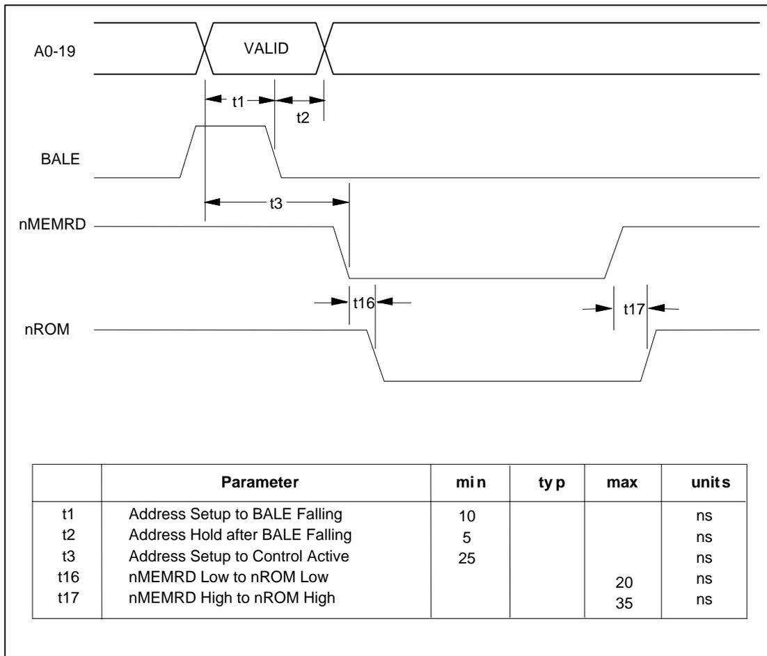
**Figure 12.14 – External ROM Read Access Using Bale**
