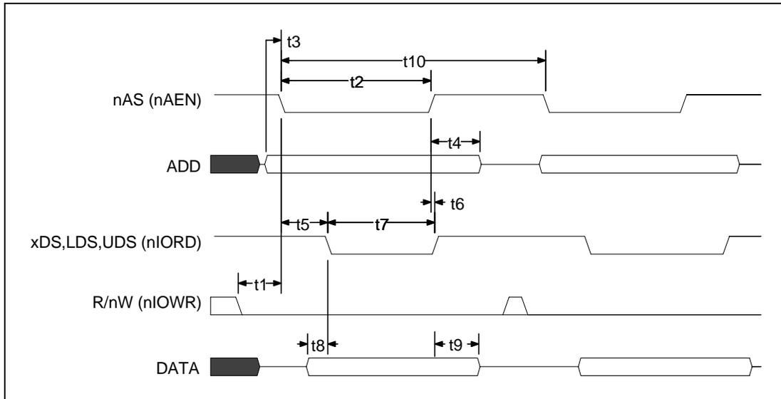
Figure 12.11 - 68000 Write Timing
