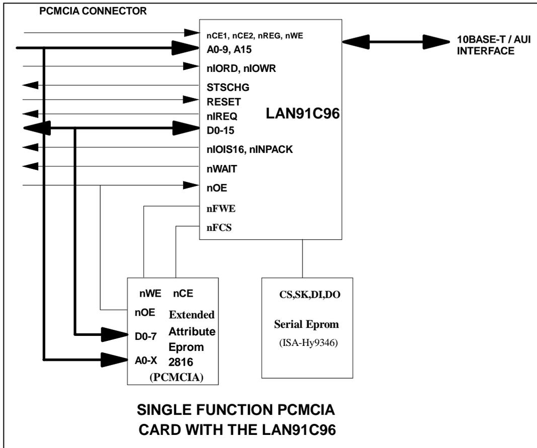
Figure 3.3 - LAN91C96 System Block Diagram
