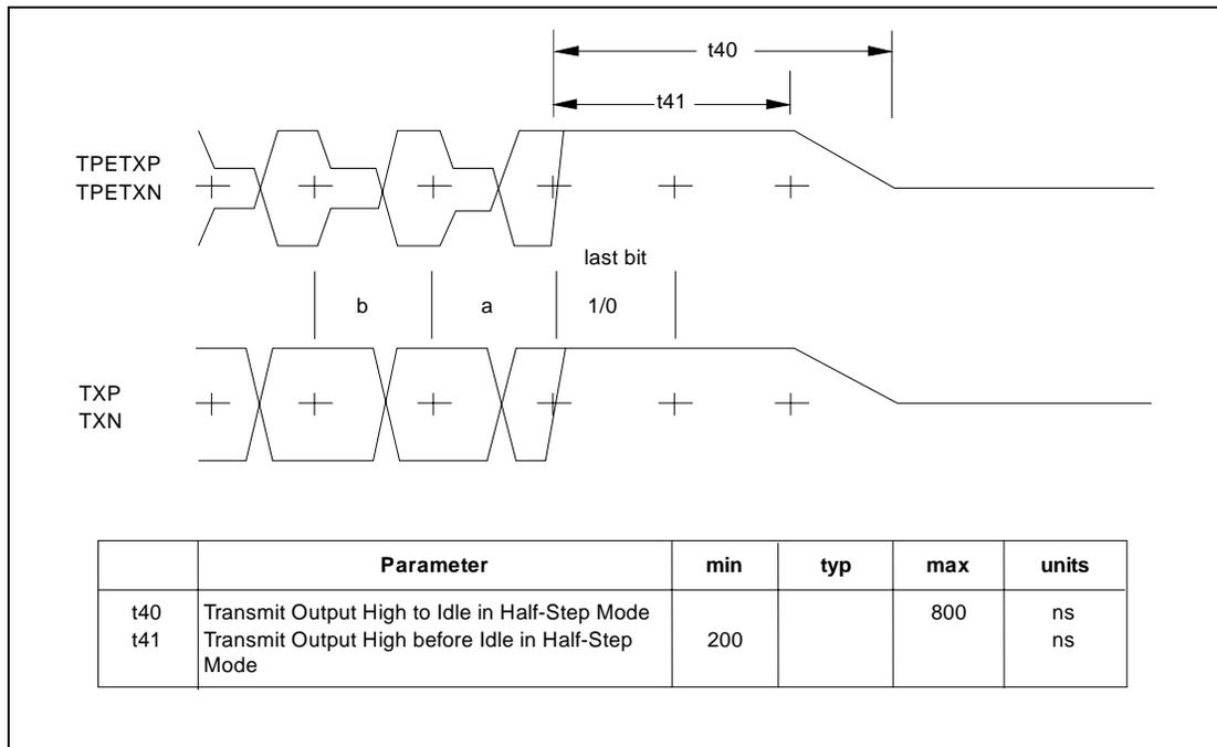
**Figure 12.23 – Transmit Timing – End of Frame (AUI and 10BASE-T)**
