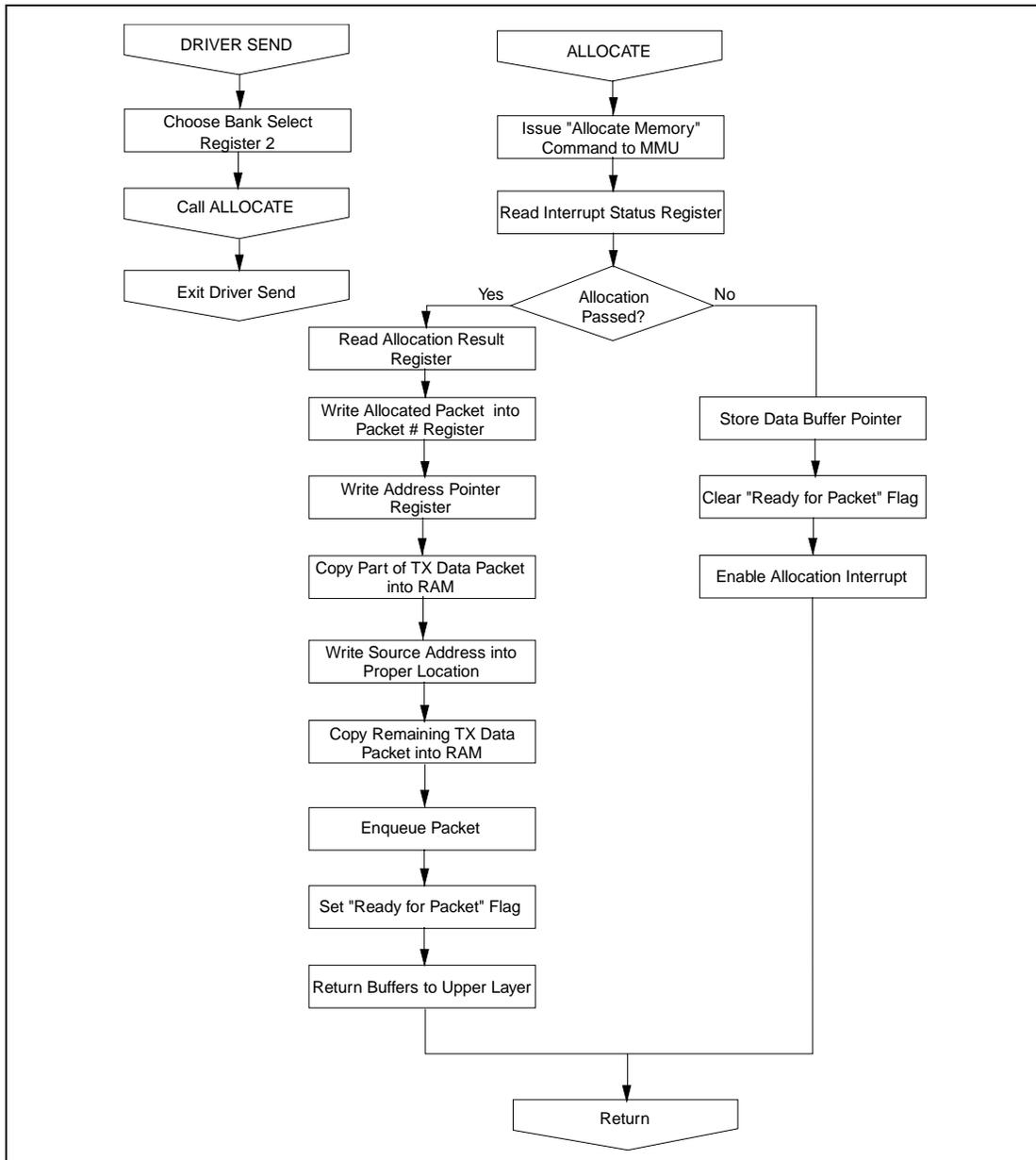
**Figure 8.5 – Driver Send and Allocate Routines**
