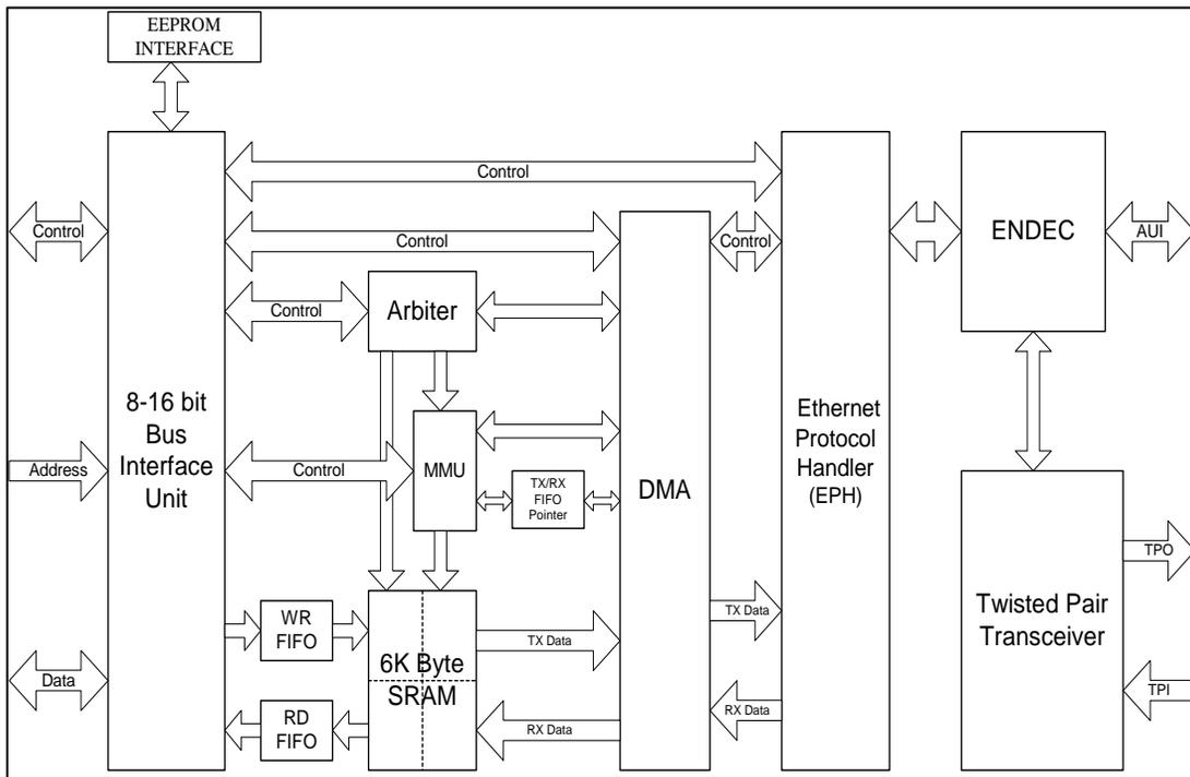
**Figure 5.4 - LAN91C96 Internal Block Diagram with Data Path**
