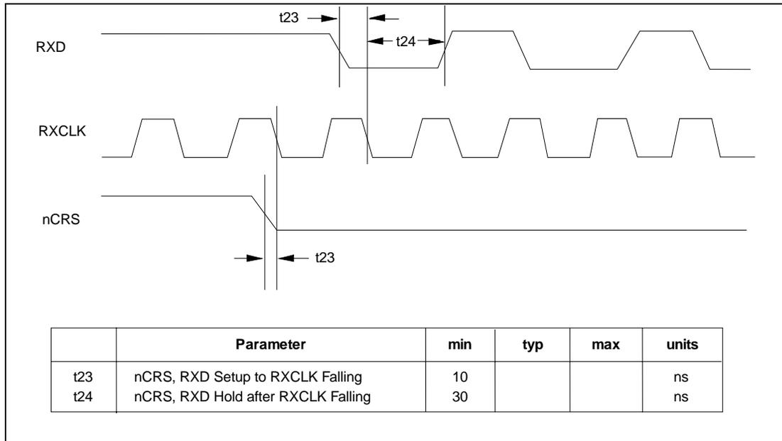
**Figure 12.19 – External ENDEC Interface – Receive Data**
