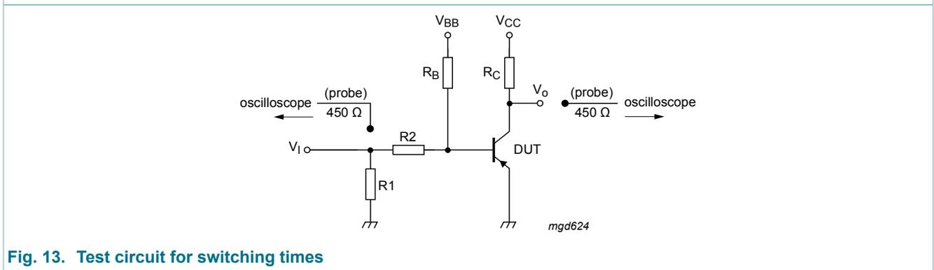
Fig. 13. Test circuit for switching times
