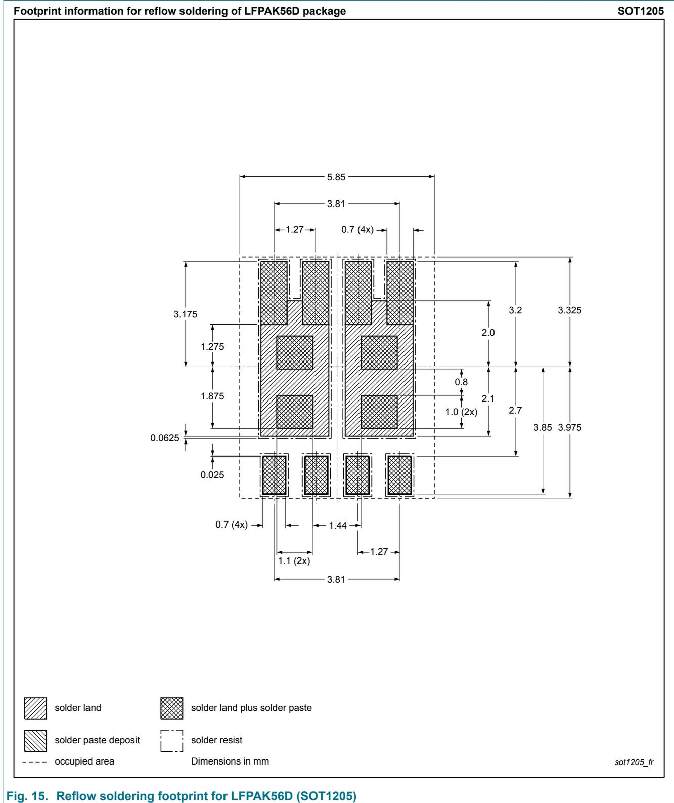
Fig. 15. Reflow soldering footprint for LFPAK56D (SOT1205)
