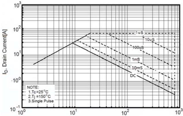
Figure2. Safe operating area for TO-220F
