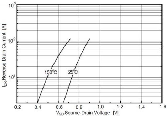
Figure4. Output characteristics
