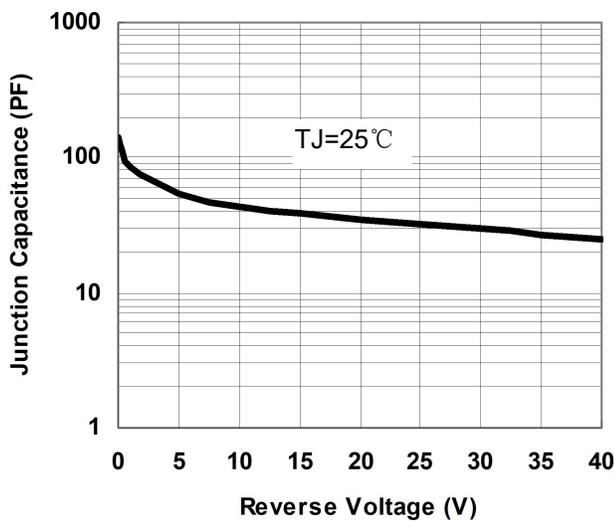
Fig.1-Typical Junction Capacitance
