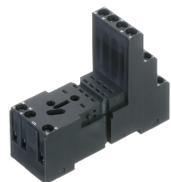
Relay socket base PRS, for industrial relay with 4 CO contacts, Screw connection, Plug-in option for input/suppression modules, Mounting type: Mounting rail TS 35
