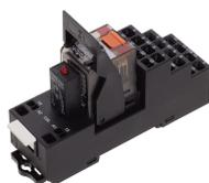
Pre-assembled relay module PRS..., Tension-spring connection, Consisting of: relay socket base, power contact relay, pluggable display/suppression module and holding clip, 4 CO contact, Input voltage: 115 VAC
