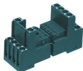
Relay socket base PRS, for industrial relay with 4 CO contacts, Screw connection, Plug-in option for input/suppression modules, Mounting type: Mounting rail TS 35
