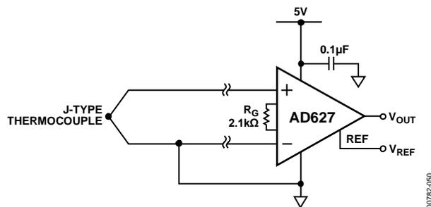
Figure 51. Amplifying Bipolar Signals with Low Common-Mode Voltage
