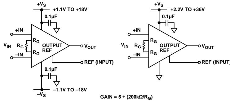
Figure 36. Basic Connections for Single and Dual Supplies
