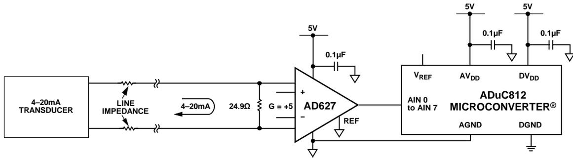
Figure 52. 4 mA to 20 mA Receiver Circuit
