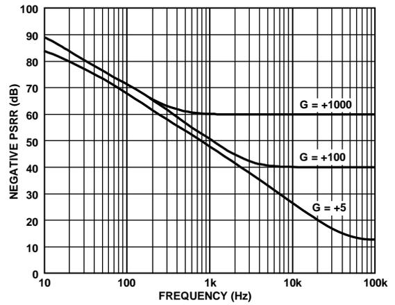
Figure 15. Negative PSRR vs. Frequency, ±5 V
