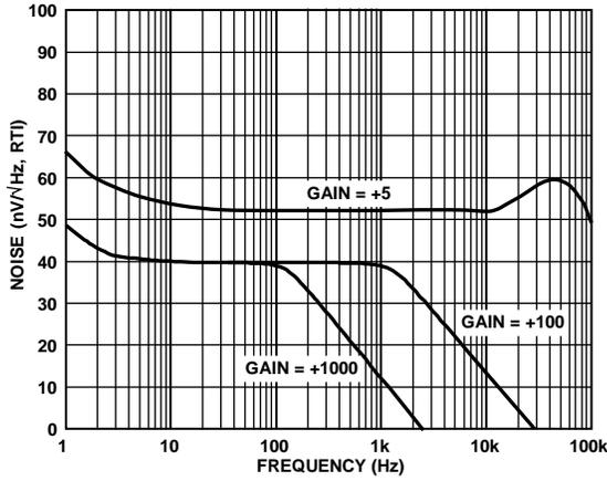
Figure 5. Voltage Noise Spectral Density vs. Frequency
