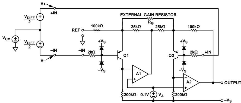
Figure 37. Amplifying Differential Signals with a Common-Mode Component
