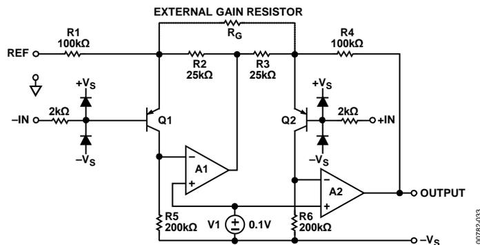
Figure 35. Simplified Schematic
