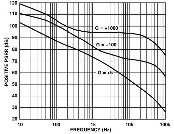
Figure 14. Positive PSRR vs. Frequency, ±5 V
