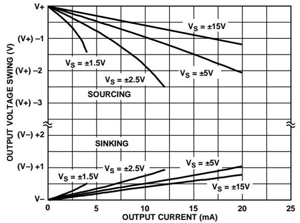
Figure 10. Output Voltage Swing vs. Output Current
