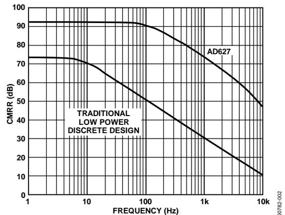
Figure 2. CMRR vs. Frequency,  $\pm$ 5 V<sub>s</sub>, Gain = +5
