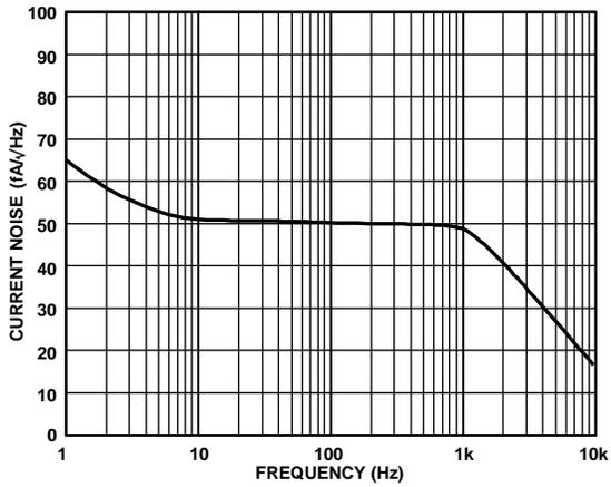
Figure 6. Current Noise Spectral Density vs. Frequency
