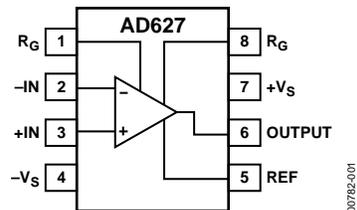
Figure 1. 8-Lead PDIP (N) and SOIC\_N (R)
