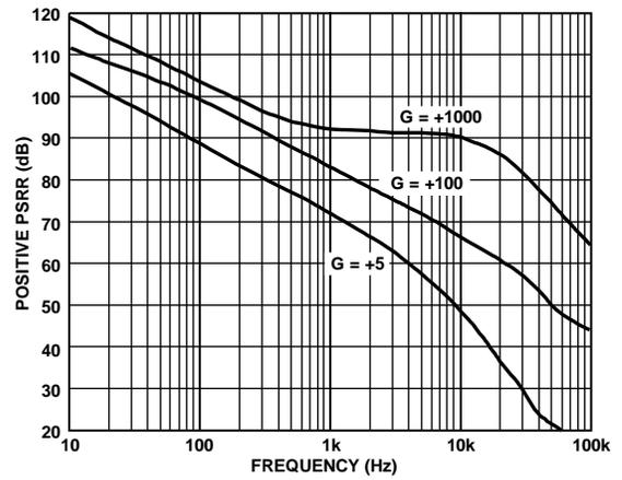
Figure 16. Positive PSRR vs. Frequency ( $V_s = 5 V, 0 V$ )
