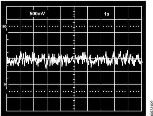
Figure 11. 0.1 Hz to 10 Hz Current Noise (0.71 pA/DIV)
