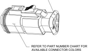
PLUG,3 SOCKET,AT,STRAIN RELIEF,REDUCED DIA WIRE SEAL
