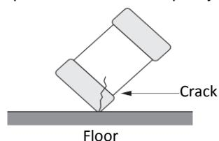
3. When printed circuit boards are piled up or handled, the corner of another printed circuit board should not be allowed to hit the capacitor, in order to avoid a crack or other damage to the capacitor.
