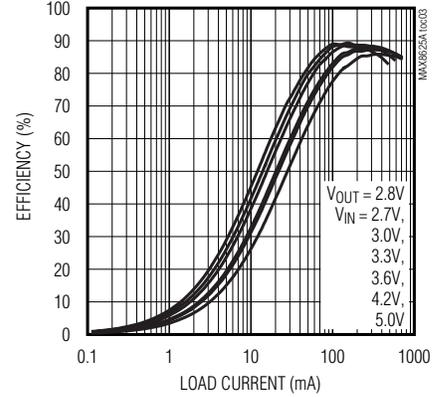
**EFFICIENCY vs. LOAD CURRENT FPWM MODE (FIGURE 3)**
