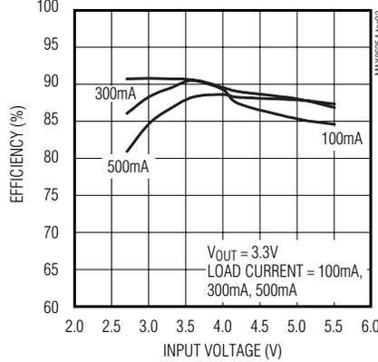
**EFFICIENCY vs. LOAD CURRENT FPWM MODE (FIGURE 3)**
