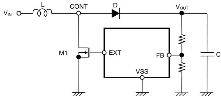
**Figure 9 Step-up Switching Regulator Circuit for Basic Equations**
