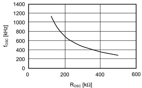
**Figure 11 R<sub>osc</sub> vs. f<sub>osc</sub>**
