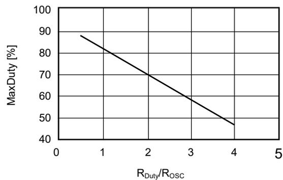
**Figure 12 R<sub>Duty</sub>/R<sub>osc</sub> vs. MaxDuty**
