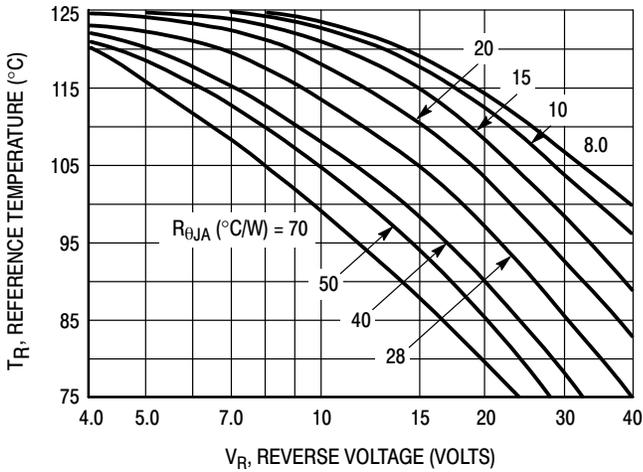
Figure 3. Maximum Reference Temperature
