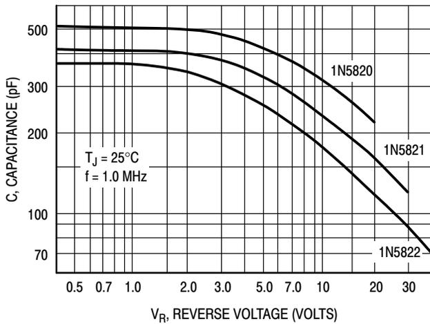
**Figure 10. Typical Capacitance**
