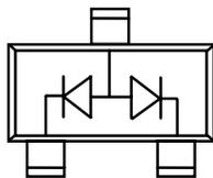
**150mW High Speed Switching Diodes
