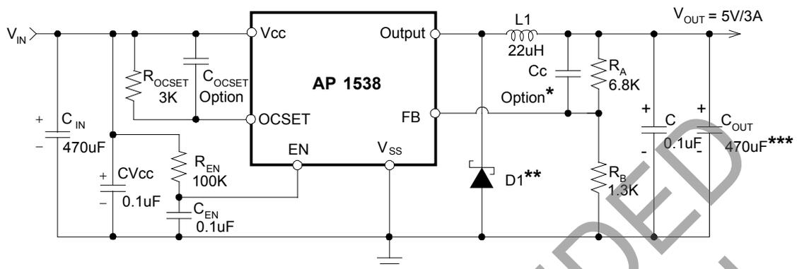
$$V_{OUT} = V_{FB} \times (1 + R_A/R_B)$$
