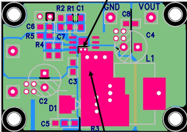
Recommended exposed-pads gap: 30~40mil (0.75~1mm)
