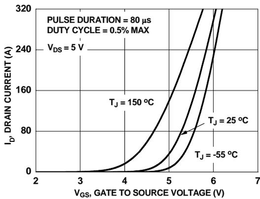
Figure 5. Transfer Characteristics
