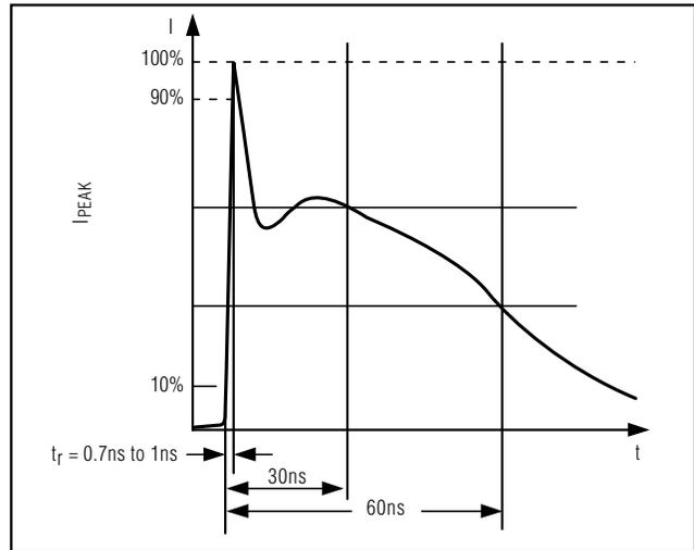
Figure 4b. IEC 1000-4-2 ESD Generator Current Waveform
