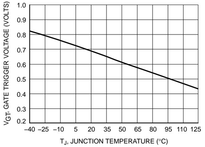
**Figure 6. Typical Gate Trigger Voltage versus Junction Temperature**
