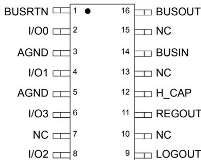
**Figure 3. 33793 Pin Connections**
