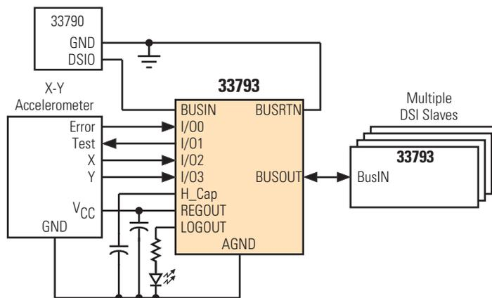
Figure 1. 33793 Simplified Application Diagram
