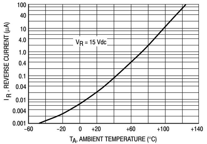
Figure 4. Leakage Current
