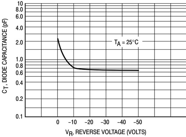
Figure 3. Diode Capacitance
