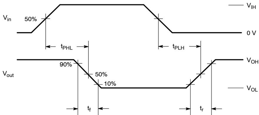
Figure 2. Switching Waveforms
