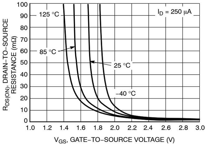
**Figure 10. On Resistance Variation vs. Gate-to-Source Voltage**
