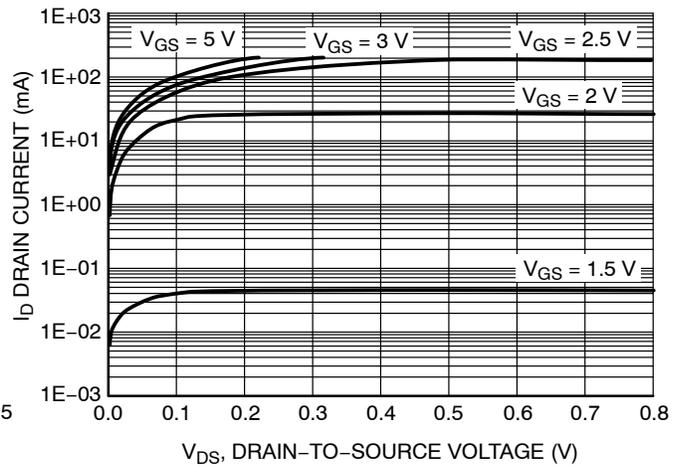
**Figure 7. Output Characteristics**
