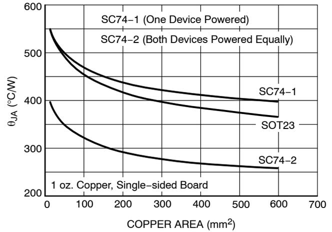
**Figure 13. Thermal Performance vs. Board Copper Area**
