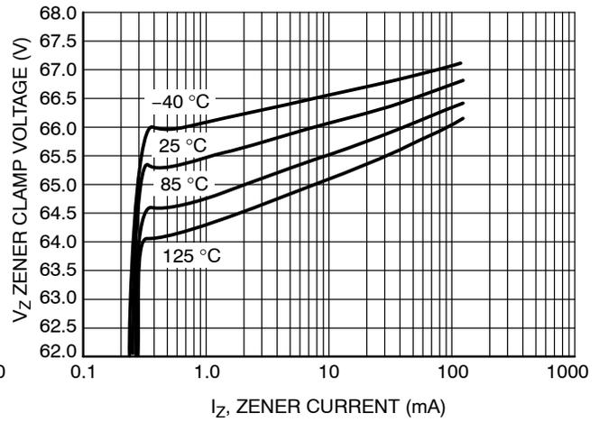
**Figure 11. Zener Clamp Voltage vs. Zener Current**
