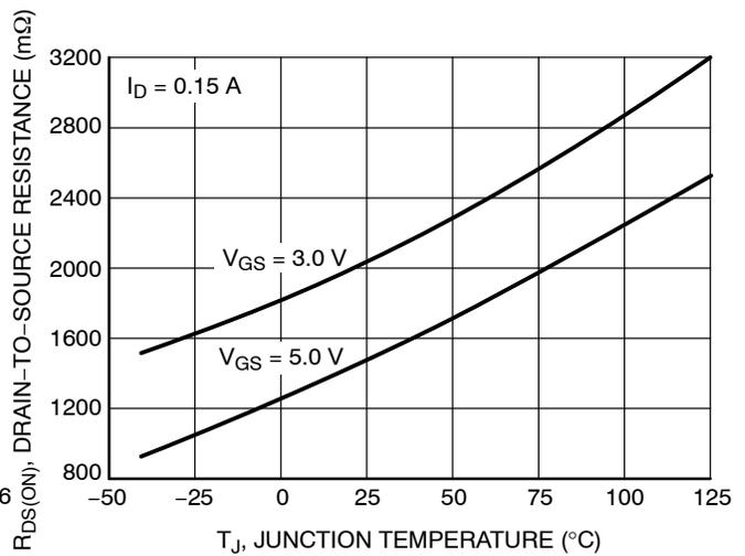
**Figure 9. On Resistance Variation vs. Junction Temperature**
