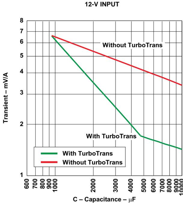
Figure 8. Capacitor Type C, 5000 < C(µF)×ESR(mΩ) ≤ 10,000(e.g. OS-CON)
