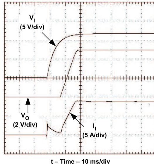
Figure 11. Power-Up Waveform
