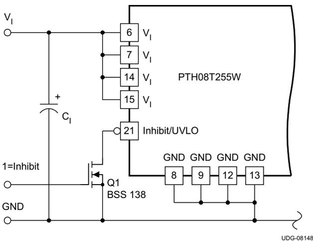
Figure 12. On/Off Inhibit Control Circuit
