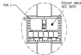
NOTE: THE INDUCTOR IS USED TO PICK AND PLACE THE MODULE. IT'S LOCATION MAY VARY FROM PACKAGE STYLE. SEE PRODUCT TABLE
