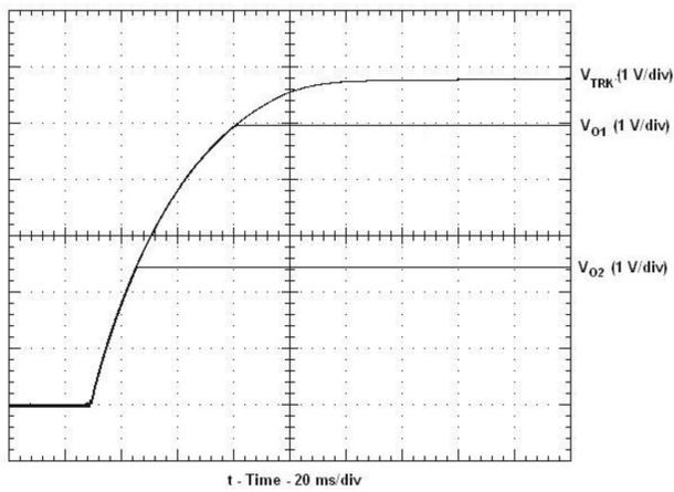
**Figure 16. Simultaneous Power Up With Auto-Track Control**
