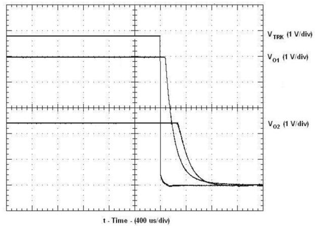
**Figure 17. Simultaneous Power Down With Auto-Track Control**
