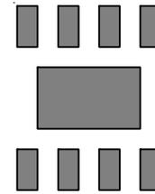
(b) Copper Area =  $10 \text{ mm}^2$ ,  $\theta_{JA} = 64^\circ\text{C/W}$
