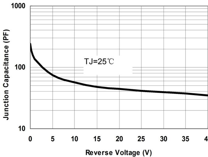
**Fig.1-Typical Junction Capacitance**
