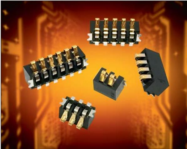
AVX extends their board-to-board right angle connectors with a new 2mm pitch version 9155-700, an addition to the existing versions 9155-300 with a 3mm pitch and 9155-500 with a 2.5mm pitch. This new connector is offered in 2 to 6 contact positions and rated at 2 Amps for the 2-4 way versions or 1.5 Amps for the 5-6 way versions. The connector's design is small and compact in order to minimize its profile, yet remain stable while having a contact point at 2.10mm above the PCB.
