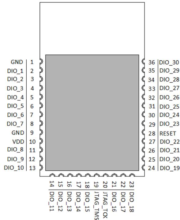
Fig. 2: The pinout of BDE-RFM206-IN (TOP VIEW)
