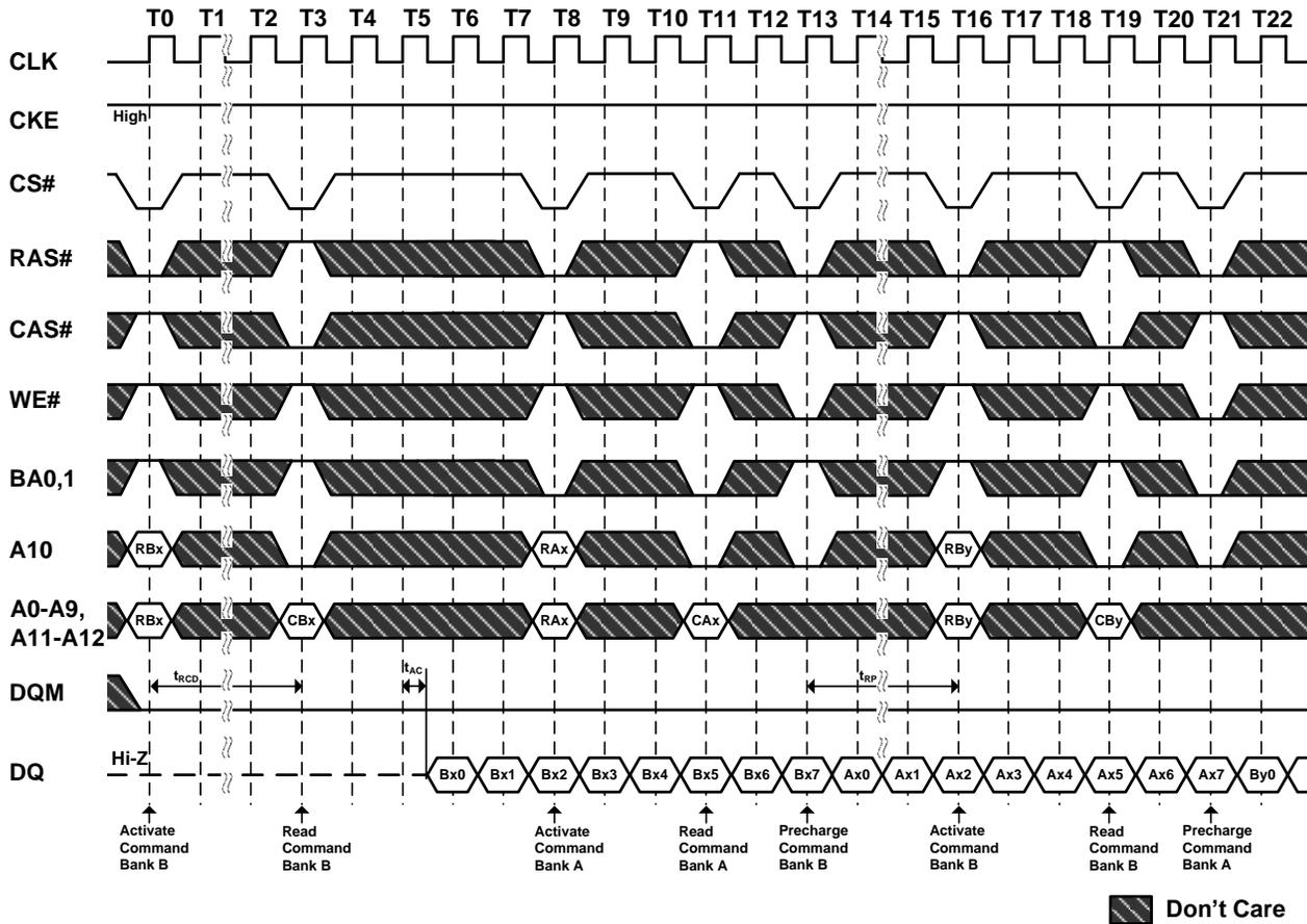
Figure 30. Random Row Write (Interleaving Banks)
