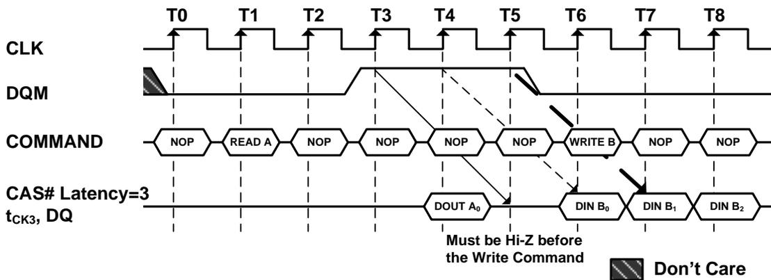
A read burst without the auto precharge function may be interrupted by a BankPrecharge/Precharge All command to the same bank. The following figure shows the optimum time that BankPrecharge/PrechargeAll command is issued in different CAS latency.
