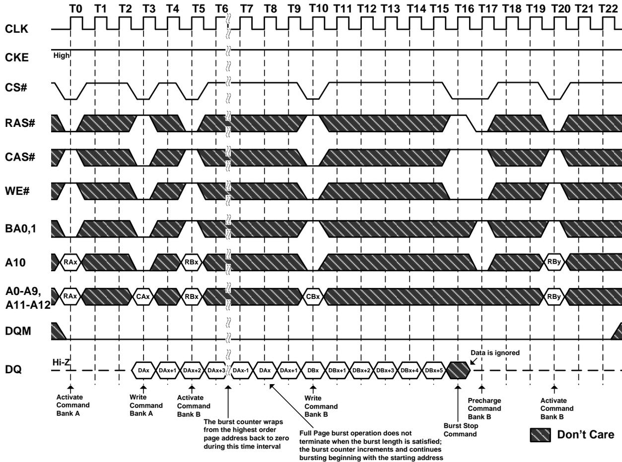
**Figure 38. Byte Read and Write Operation**
