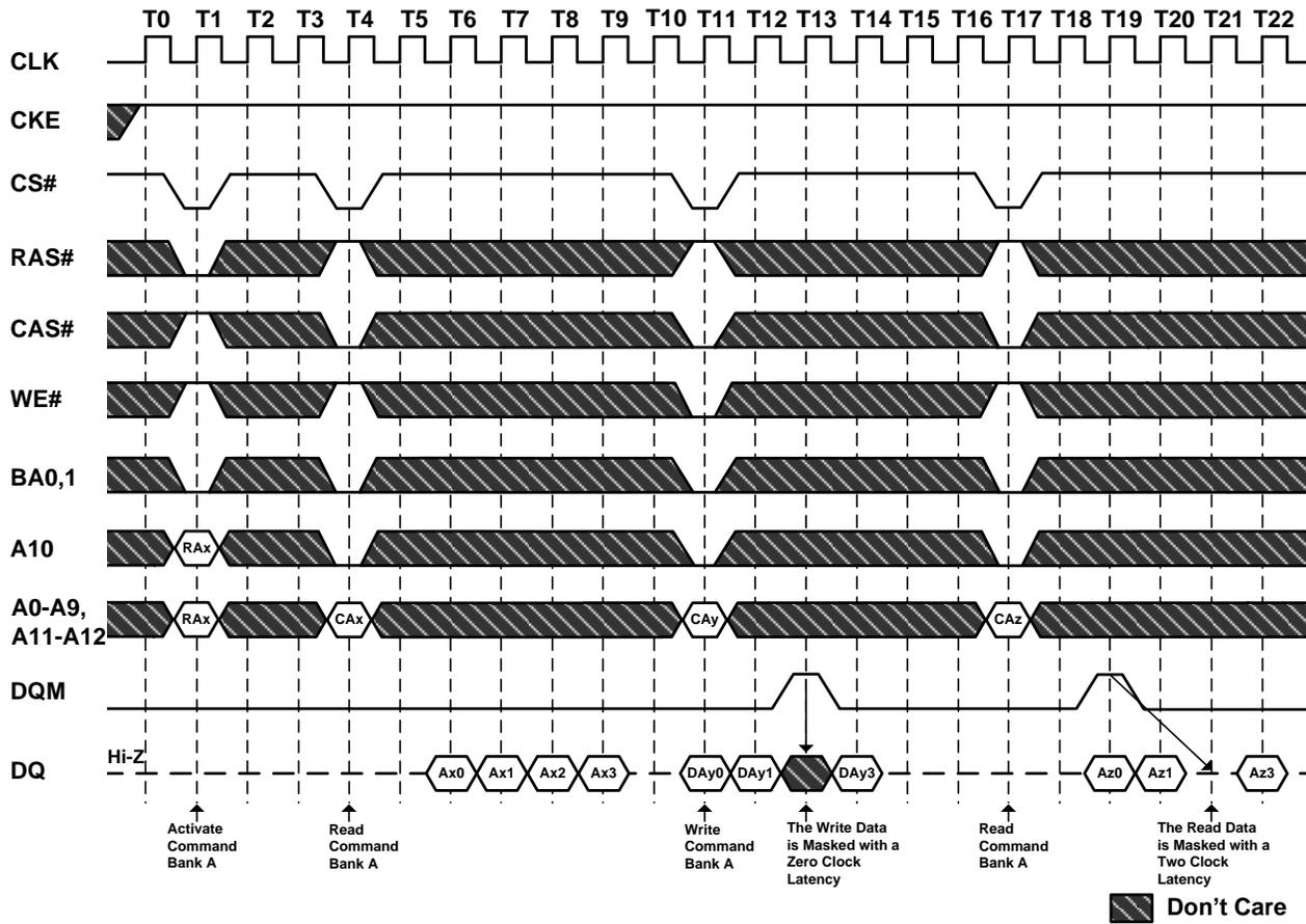
**Figure 31.2. Read and Write Cycle**
