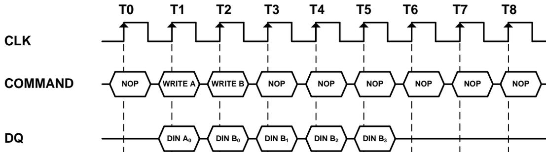
The Read command that interrupts a write burst without auto precharge function should be issued one cycle after the clock edge in which the last data-in element is registered. In order to avoid data contention, input data must be removed from the DQs at least one clock cycle before the first read data appears on the outputs (refer to the following figure). Once the Read command is registered, the data inputs will be ignored and writes will not be executed.
