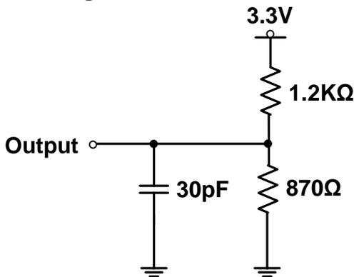
**Figure 18.2 LVTTL A.C. Test Load (B)**
