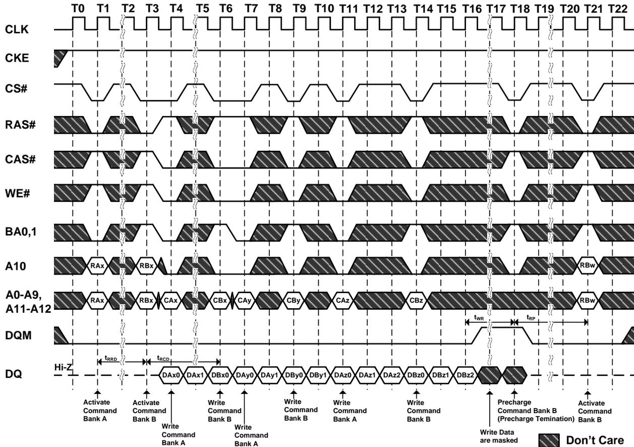
**Figure 42. Precharge Termination of a Burst**
