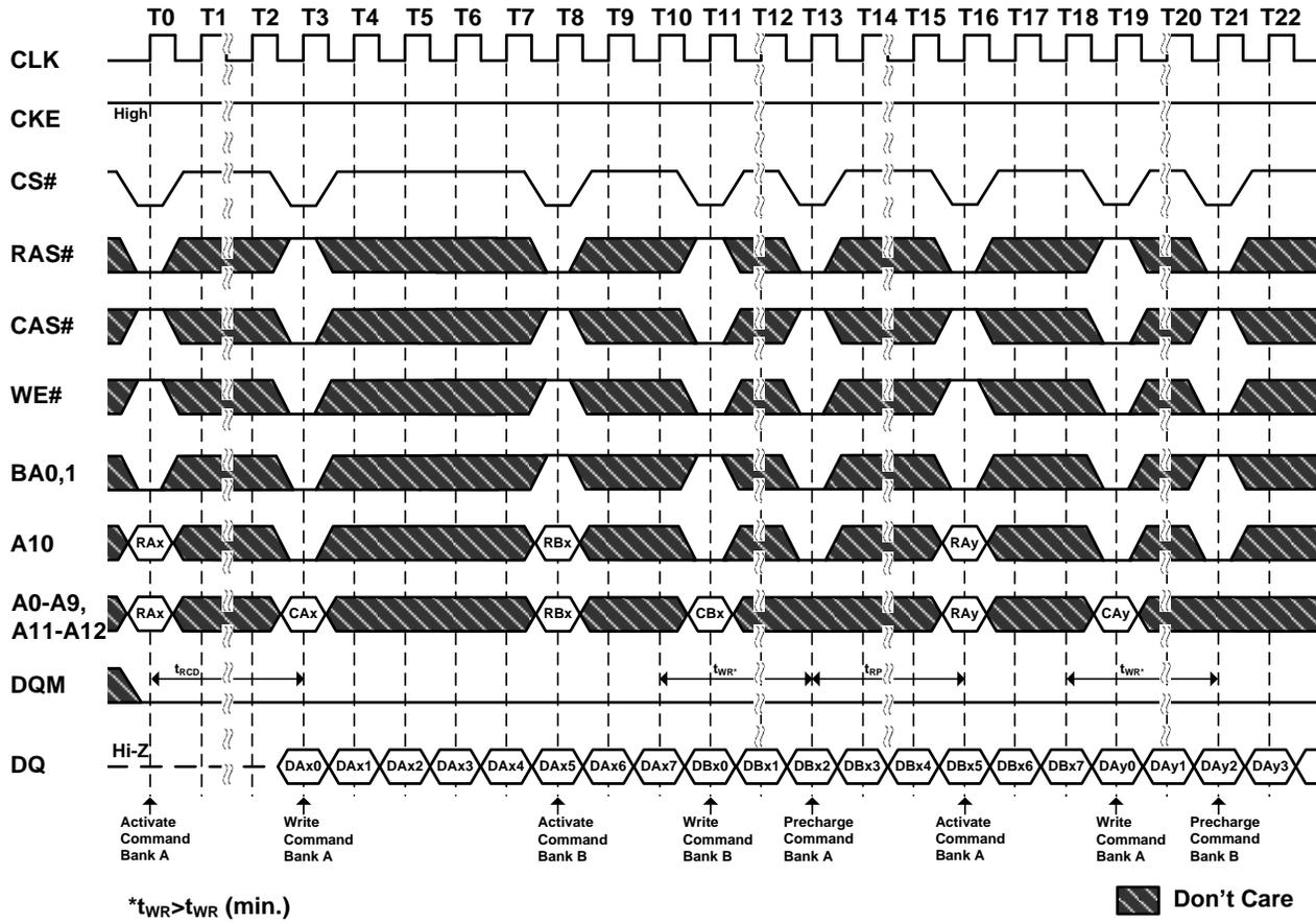
**Figure 31.1. Read and Write Cycle**
