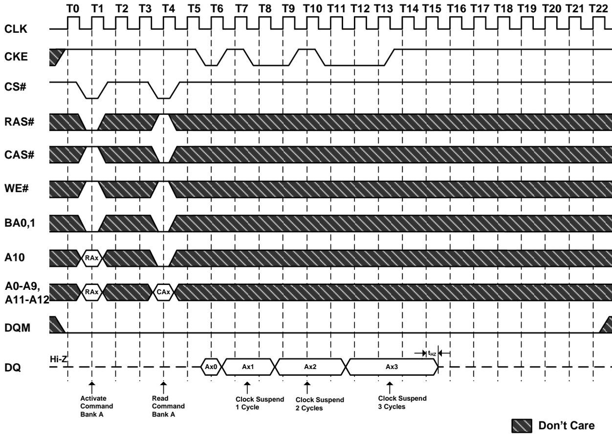
**Figure 24.2. Clock Suspension During Burst Read (Using CKE)**
