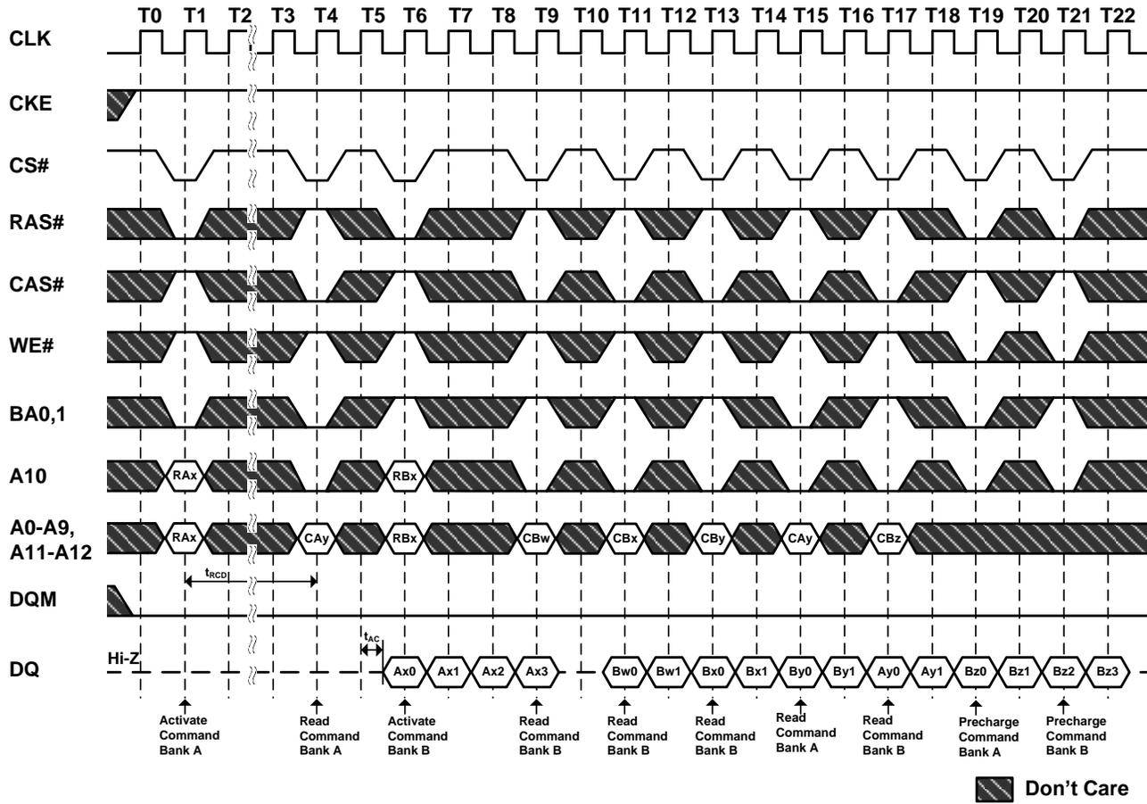
**Figure 32.2. Interleaved Column Read Cycle**
