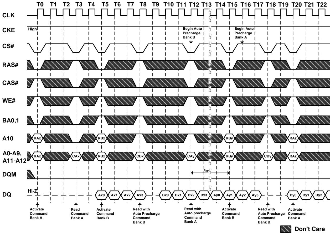
**Figure 34.2. Auto Precharge after Read Burst**
