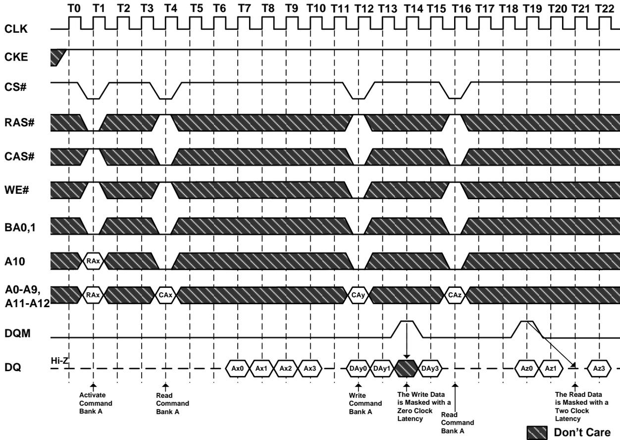
**Figure 32.1. Interleaving Column Read Cycle**
