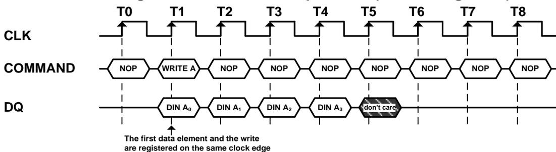
A write burst without the auto precharge function may be interrupted by a subsequent Write, BankPrecharge/PrechargeAll, or Read command before the end of the burst length. An interrupt coming from Write command can occur on any clock cycle following the previous Write command (refer to the following figure).
