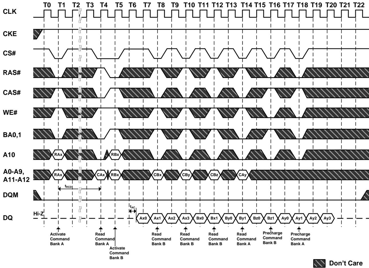
**Figure 33. Interleaved Column Write Cycle
