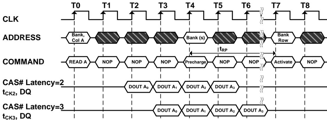
5. Read and AutoPrecharge command (RAS# = "H", CAS# = "L", WE# = "H", BAs = Bank, A10 = "H", A0-A8 = Column Address)
