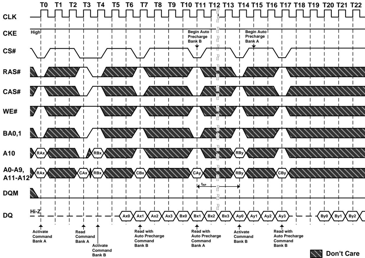
**Figure 35. Auto Precharge after Write Burst
