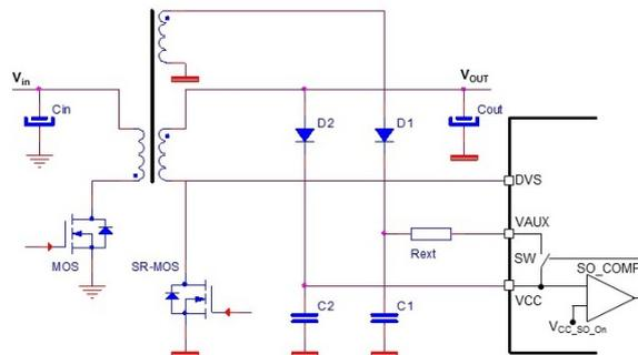
Considering the circuit in Figure 13, the following exemplification is provided to calculate the value of  $R_{ext}$  resistor and power dissipation, in the case of a +5 V charger with operation down to 2 V in CC regulation and transformer secondary-to-primary reflected voltage of 75V:
