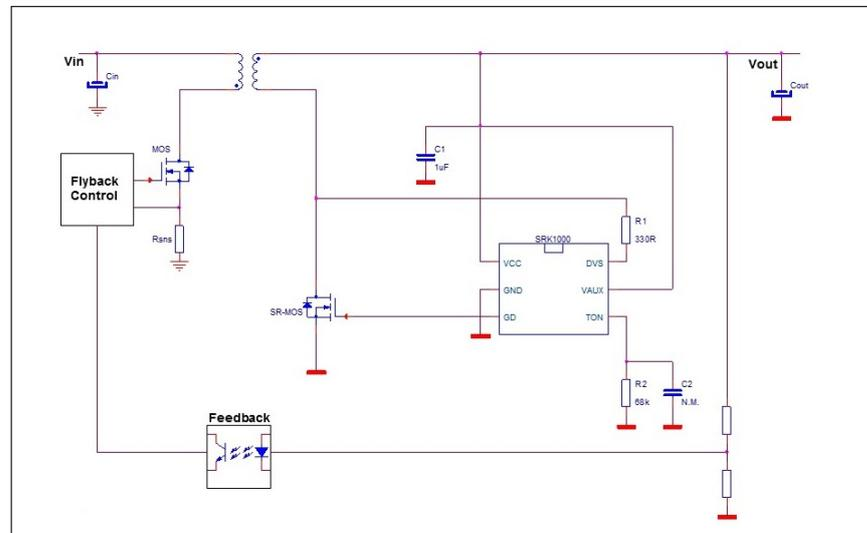
Figure 5. Fixed frequency CCM flyback adapter (CV regulation)
