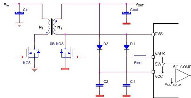
The VAUX pin may be connected, for example, to the rectified SR MOSFET drain voltage, like in Figure 13 or to another auxiliary voltage of the flyback transformer as shown in Figure 14.
