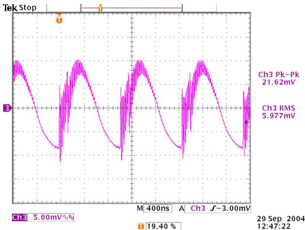
Figure 49. Output Voltage Noise, Full Load, No Interleave
