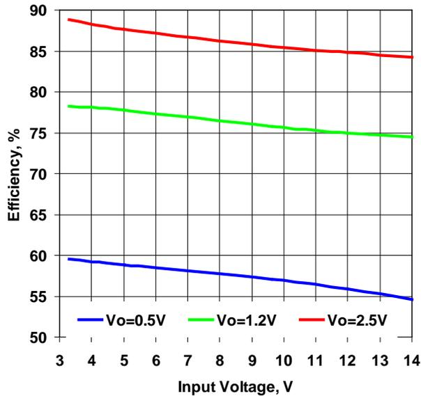
Figure 7. Efficiency vs. Input Voltage. I<sub>out</sub>=7A, F<sub>sw</sub>=500kHz
