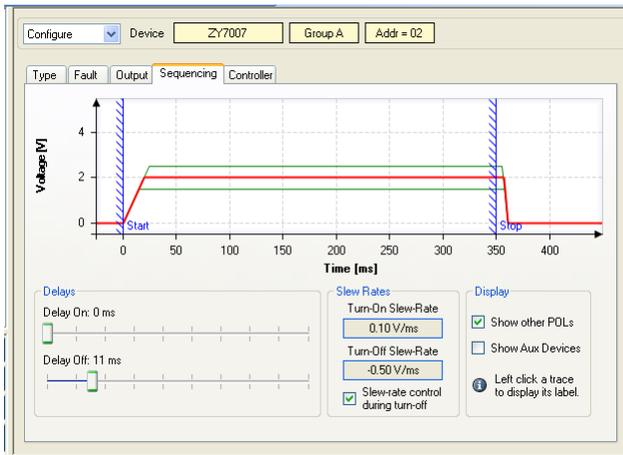
Figure 30. POL Configure Sequencing Window
