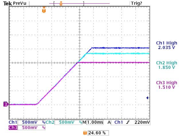
Figure 8. Tracking Turn-On. Rising Slew Rate is Programmed at 0.5V/ms.
