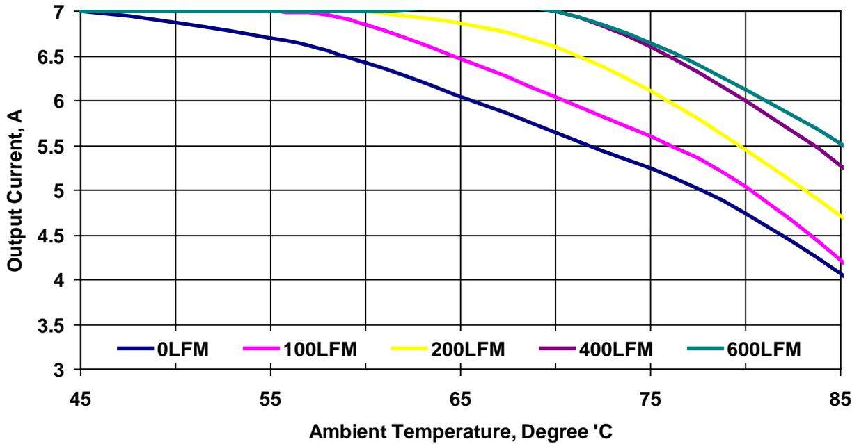
Figure 21. Thermal Derating Curves. Vin=12V, Vout=5.0V, Fsw=1MHz
