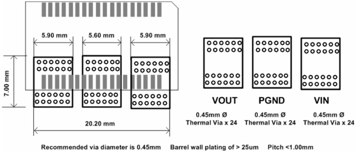
Figure 59. Recommended PCB Layout for Multilayer PCBs
