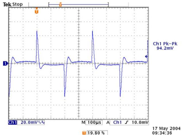
Figure 28. Transient Response without Optimal Voltage Positioning
