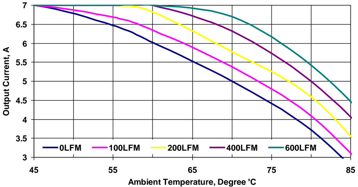
Figure 22. Thermal Derating Curves. Vin=14V, Vout=5.0V, Fsw=1MHz
