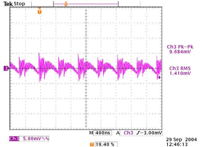
Figure 50. Output Voltage Noise, Full Load, 180° Interleave
