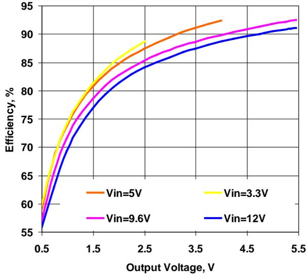
Figure 6. Efficiency vs. Output Voltage. I<sub>out</sub>=7A, F<sub>sw</sub>=500kHz
