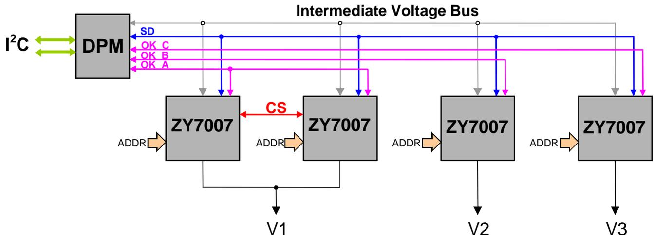
Figure 23. Block Diagram of Typical Multiple Output Application with Digital Power Manager and I<sup>2</sup>C Interface
