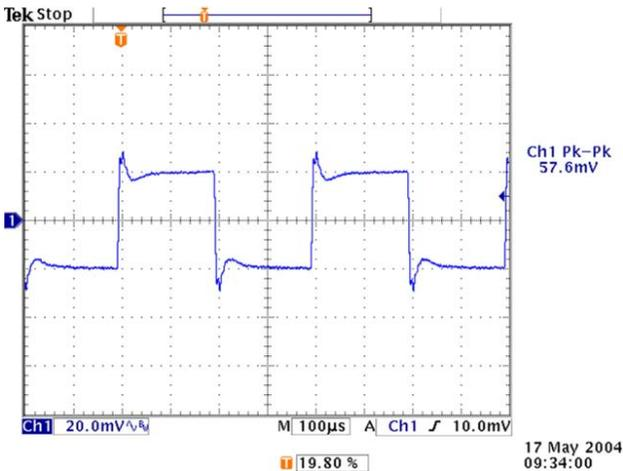
Figure 29. Transient Response with Optimal Voltage Positioning
