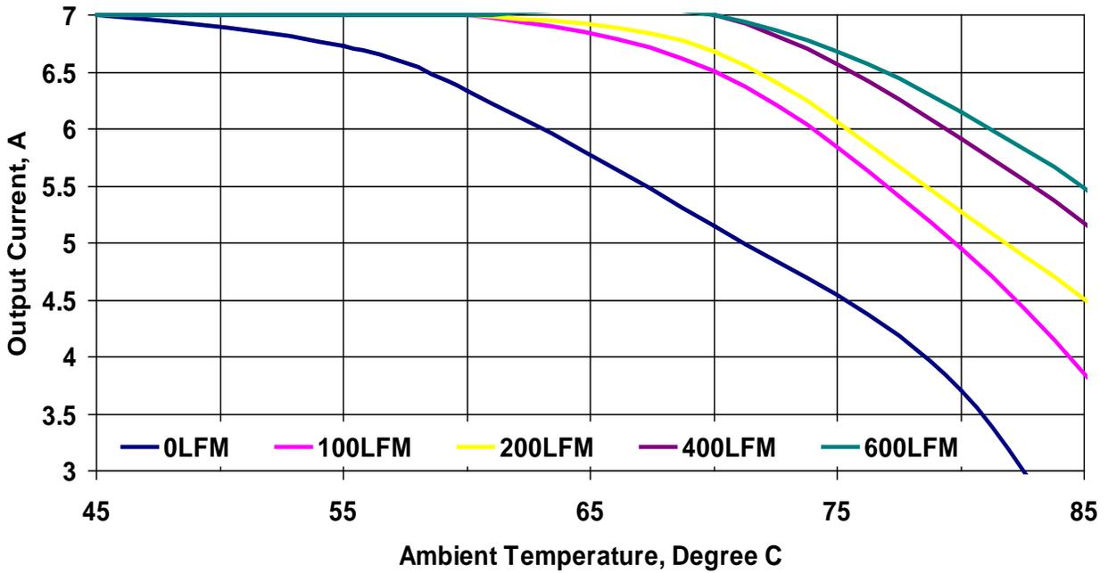
Figure 20. Thermal Derating Curves. Vin=14V, Vout=5.0V, Fsw=500kHz
