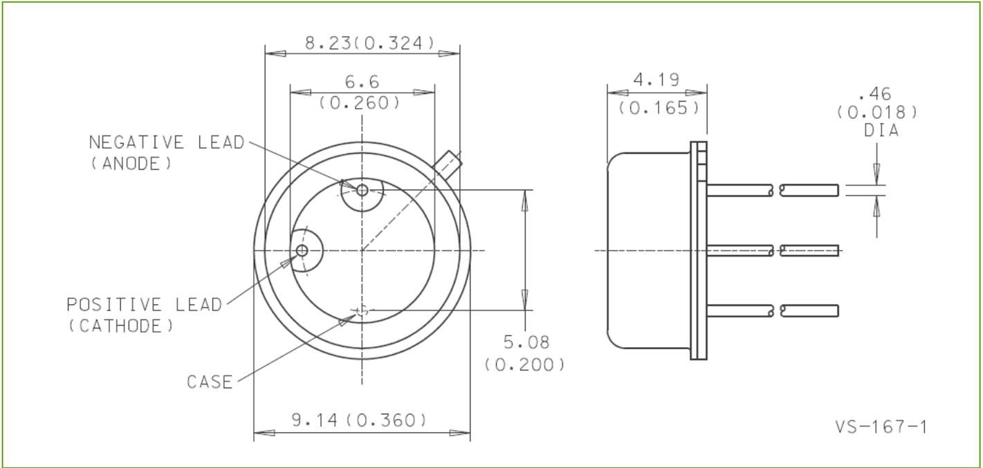
Figure 15 – Dimensional Outline (C30956EH Types) Low-Profile TO-5 Package, dimensions in mm (inch)
