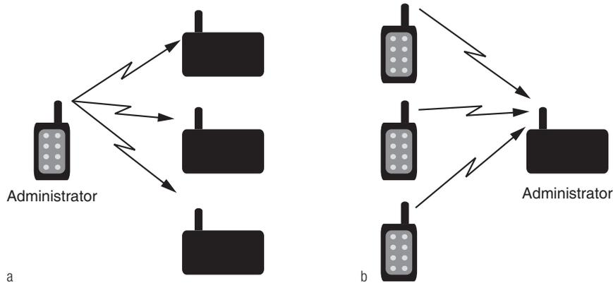
Figure 20: HumPRC™ Series Transceiver Transmitter to Receiver Ratios
