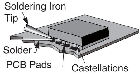
Figure 95: Soldering Technique
