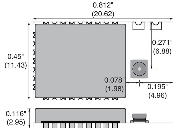
Figure 18: HumPRC™ Series Transceiver Encapsulated Version Dimensions
