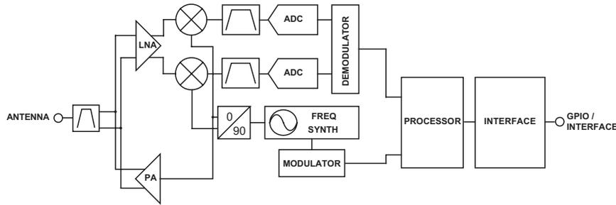
Figure 19: HumPRC™ Series Transceiver RF Section Block Diagram
