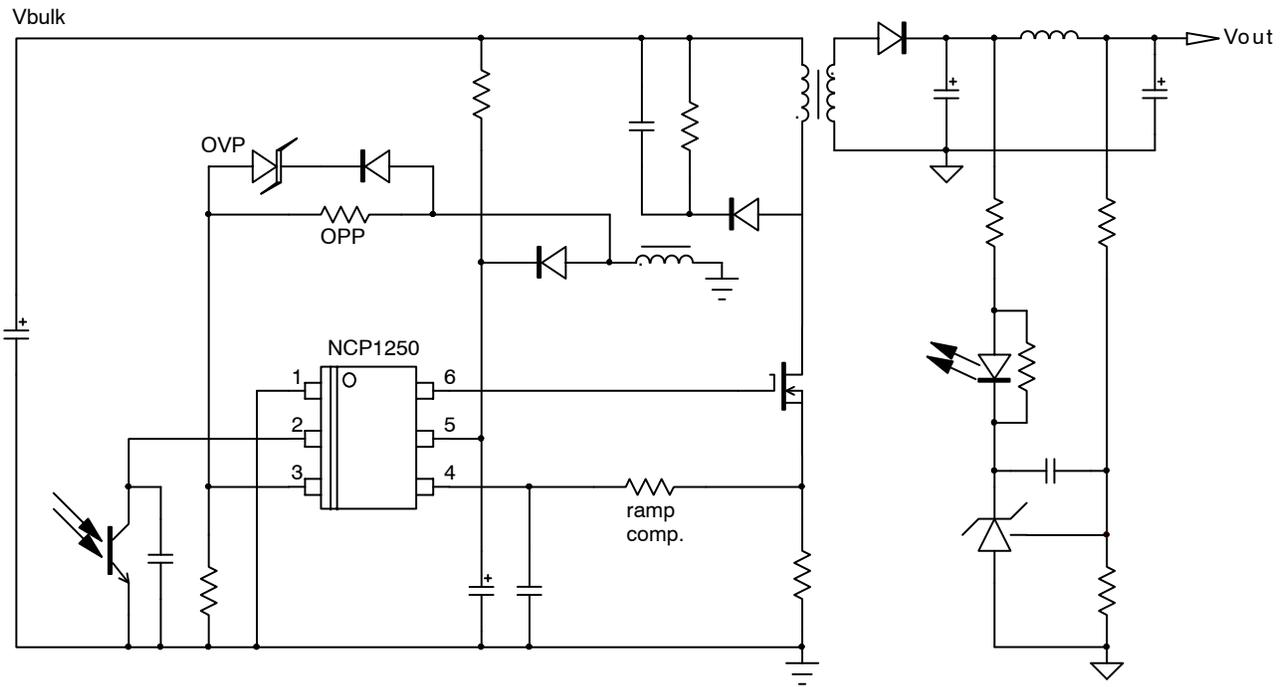
Figure 1. Typical Application Example (TSOP-6)
