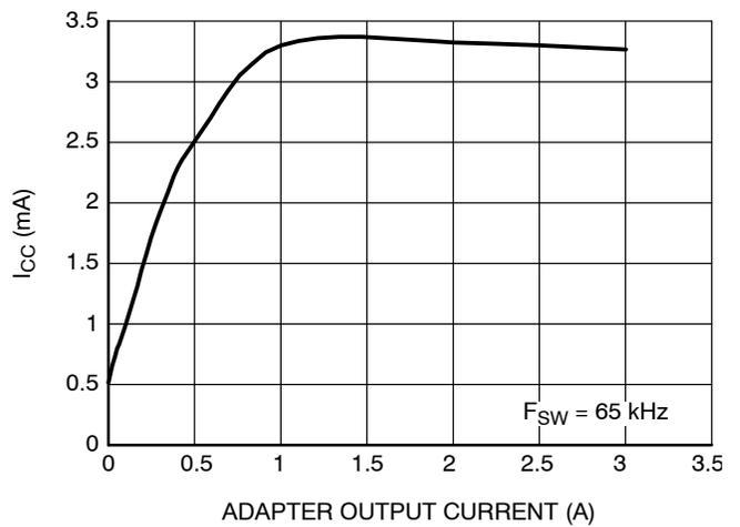
Figure 38. Controller Consumption vs. Adapter Output Current
