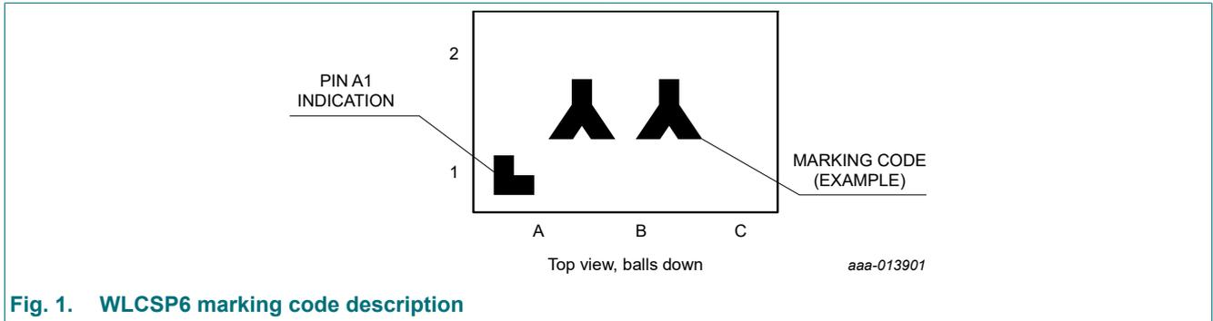
Fig. 1. WLCSP6 marking code description
