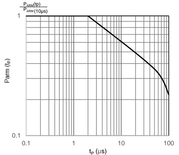
Figure 6. Normalized Avalanche Power Derating Versus Pulse Duration
