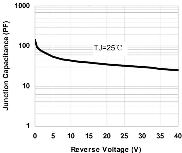
Fig.1-Typical Junction Capacitance
