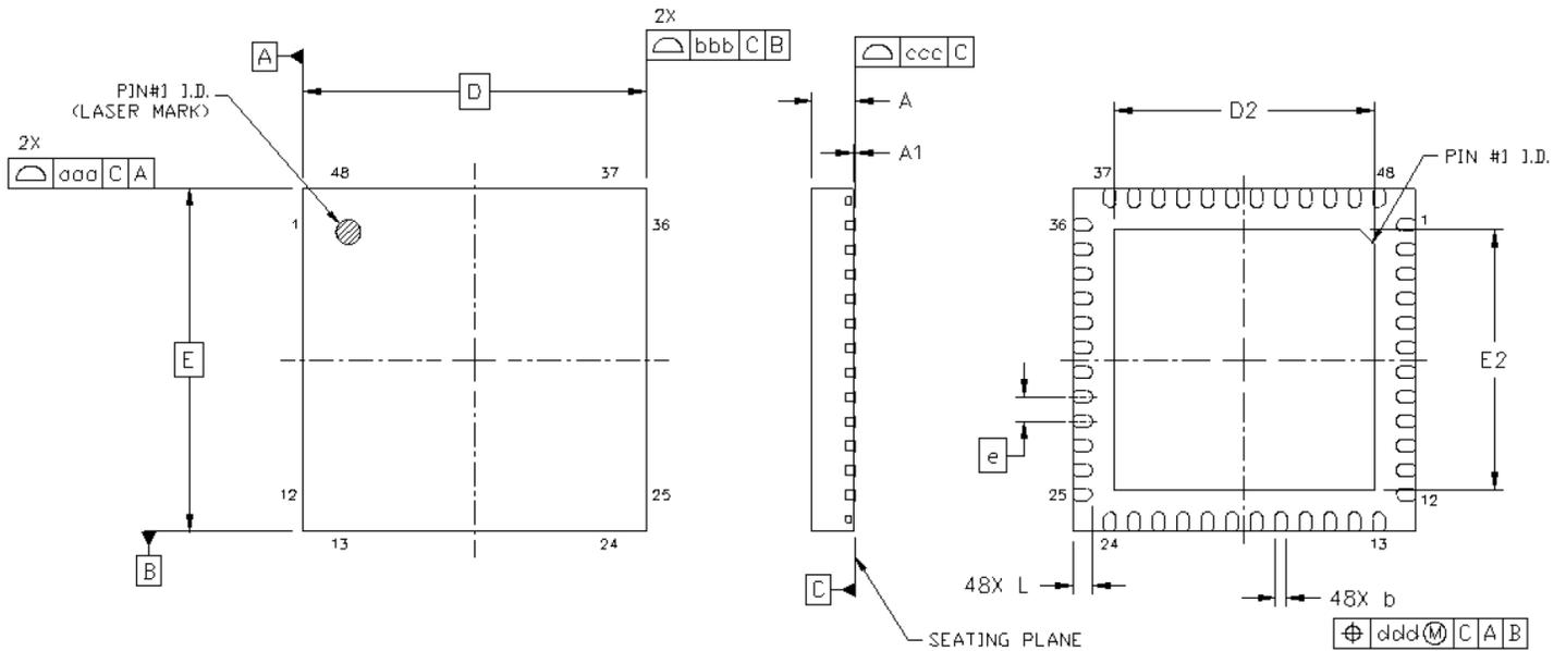
Figure 2.1. 48-Pin QFN
